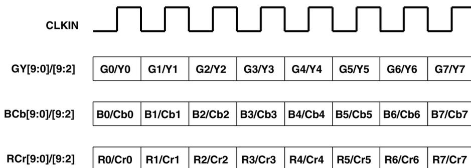
Figure 4-1. 24-/30-Bit RGB or YCbCr Data Format
