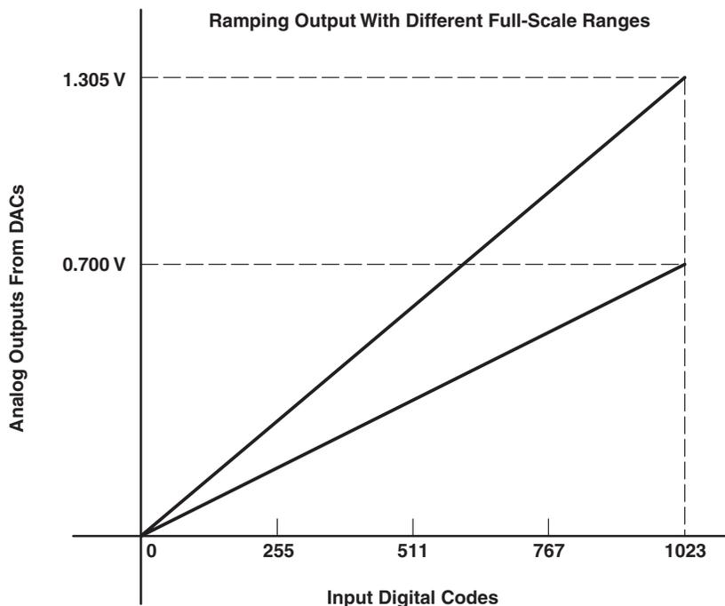
Figure 4-40. Ramping Output With Different Full-Scale Ranges
