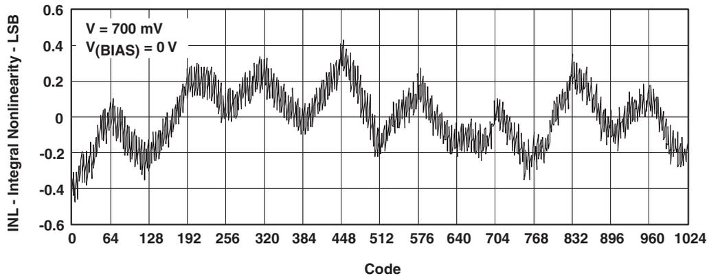
Figure 7-5. INTEGRAL NONLINEARITY vs CODE
