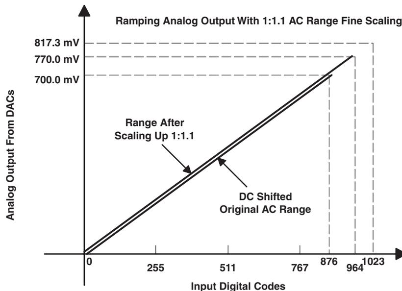
Figure 4-7. Effect of Scaling the Analog Video Output
