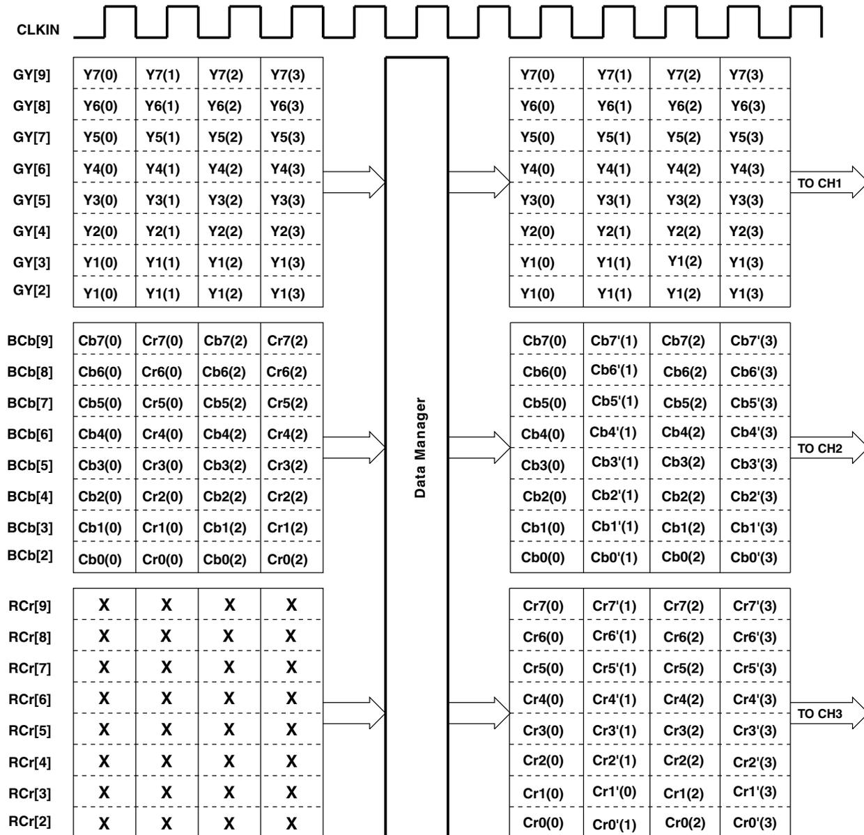
Figure 4-2. 20-/16-Bit YCbCr 4:2:2 Data Format (16-Bit Operation Shown)
