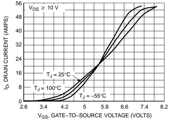
**Figure 2. Transfer Characteristics**
