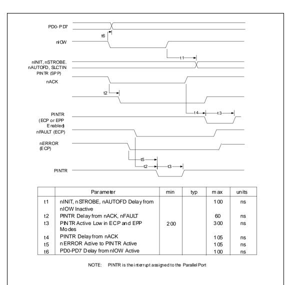
FIGURE 14 - PARALLEL PORT TIMING
