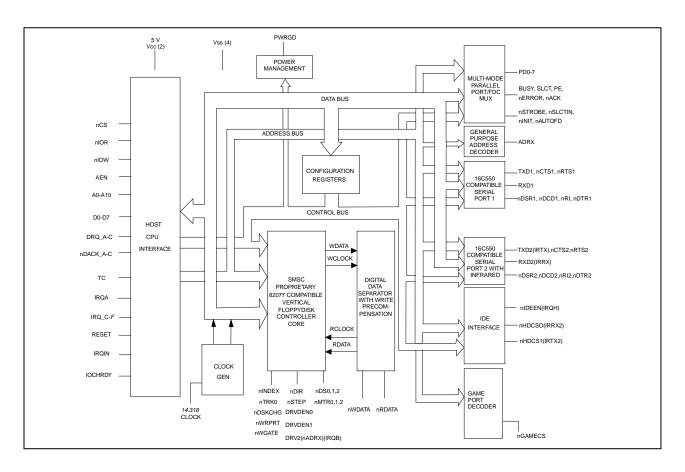
FIGURE 1 - FDC37C669 BLOCK DIAGRAM
