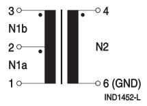
Recommendation: Connect pin 6 on PCB to GND
