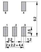
Recommended PCB layout (top view)
