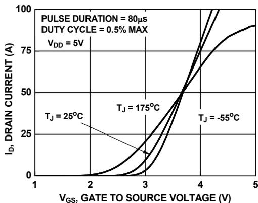
Figure 7. Transfer Characteristics
