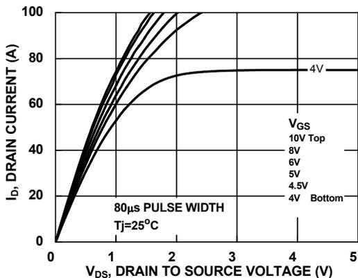
Figure 9. Saturation Characteristics
