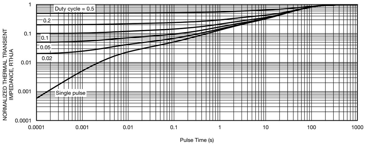
Fig. 13 - Normalized Thermal Transient Impedance, Junction-to-Ambient
