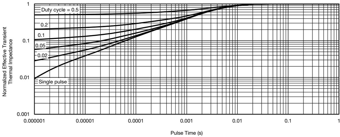
Fig. 12 - Normalized Transient Thermal Impedance, Junction-to-Case
