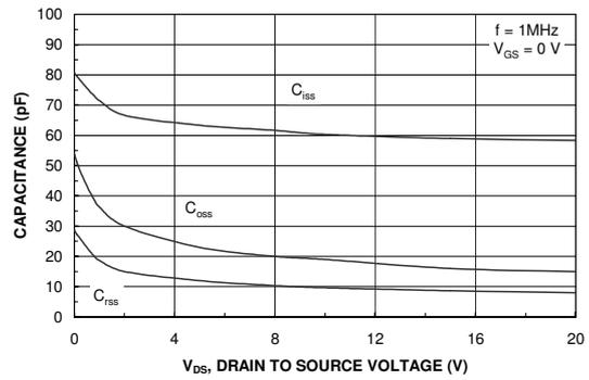
Figure 8. Capacitance Characteristics.
