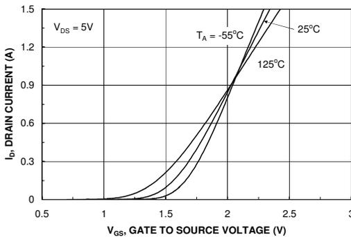
Figure 5. Transfer Characteristics.
