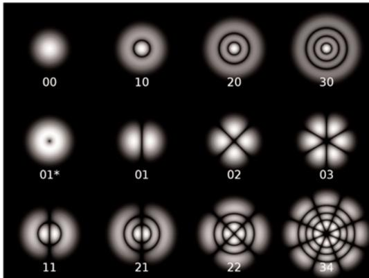
Figure 5a. Examples of Transverse Electromagnetic Modes ( $TEM_{pq}$ ).
