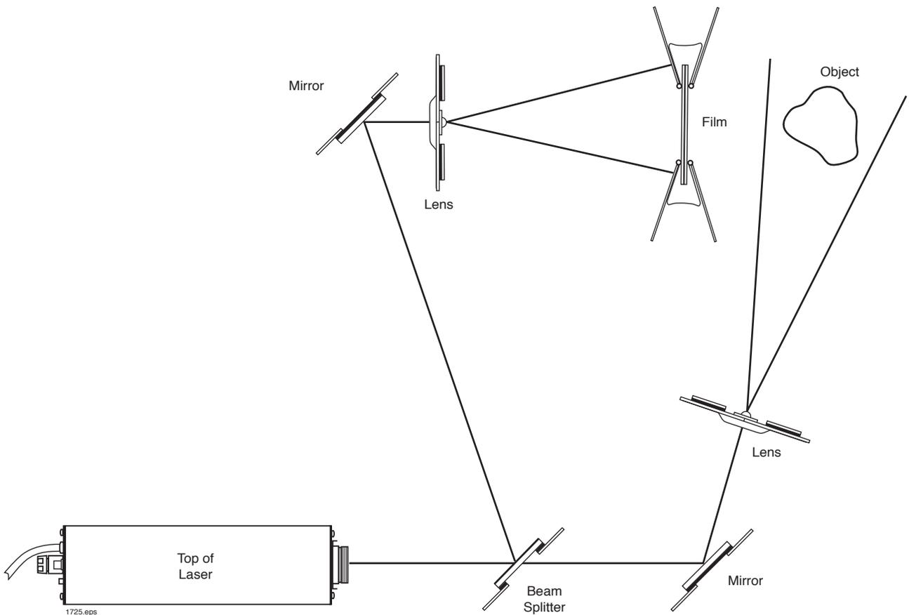
Figure 24. Setup for capturing a multiple beam reflection hologram.
