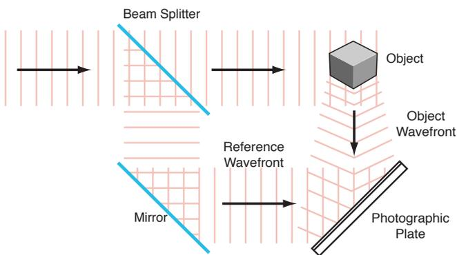
Figure 1a. Recording a hologram.
