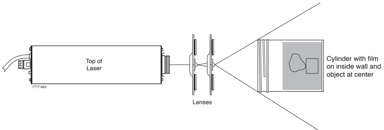
**Figure 19. Setup for capturing a 360° transmission hologram.**
