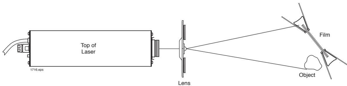
**Figure 17. Setup for capturing a direct beam transmission hologram.**
