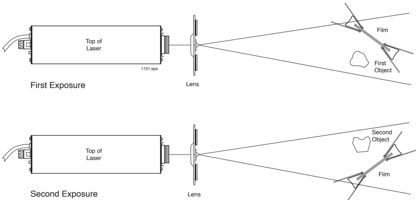
Figure 27. Setup for capturing a multiple channel transmission hologram.
