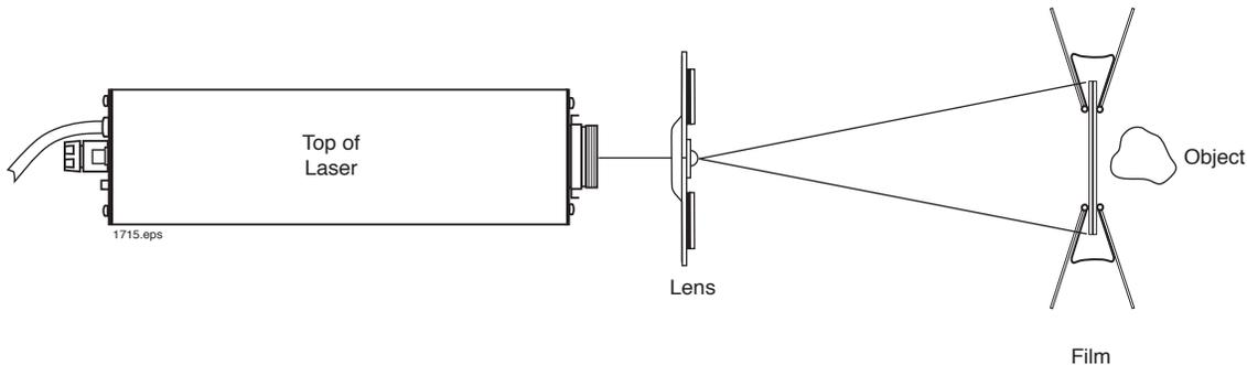
Figure 16. Setup for capturing a direct beam reflection hologram.
