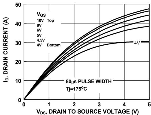
Figure 10. Saturation Characteristics
