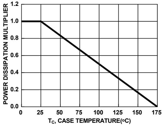
Figure 1. Normalized Power Dissipation vs Case Temperature
