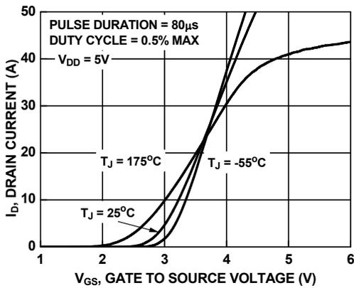
Figure 7. Transfer Characteristics
