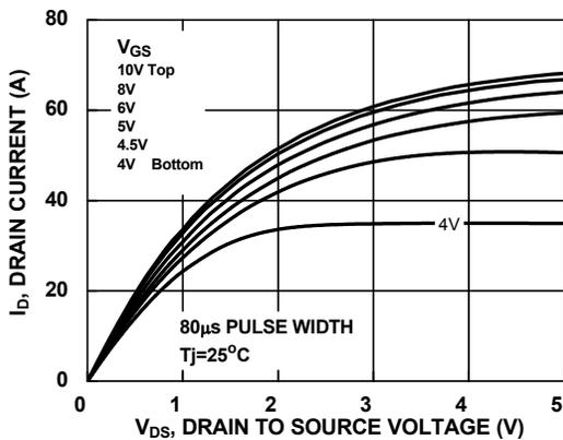
Figure 9. Saturation Characteristics
