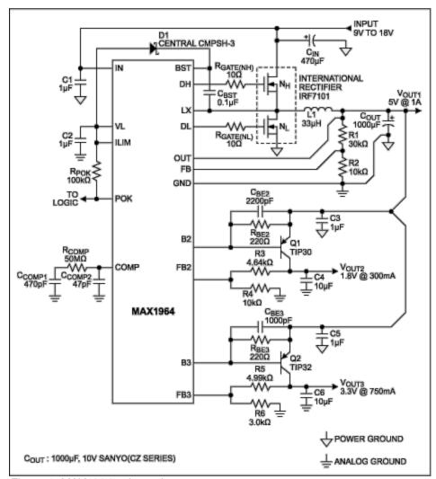
Figure 1. MAX1964 schematic.
