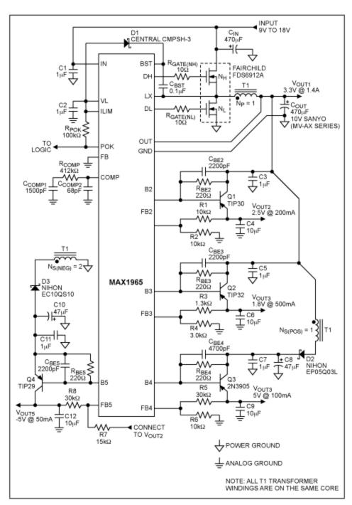
Figure 3. MAX1965 schematic.
