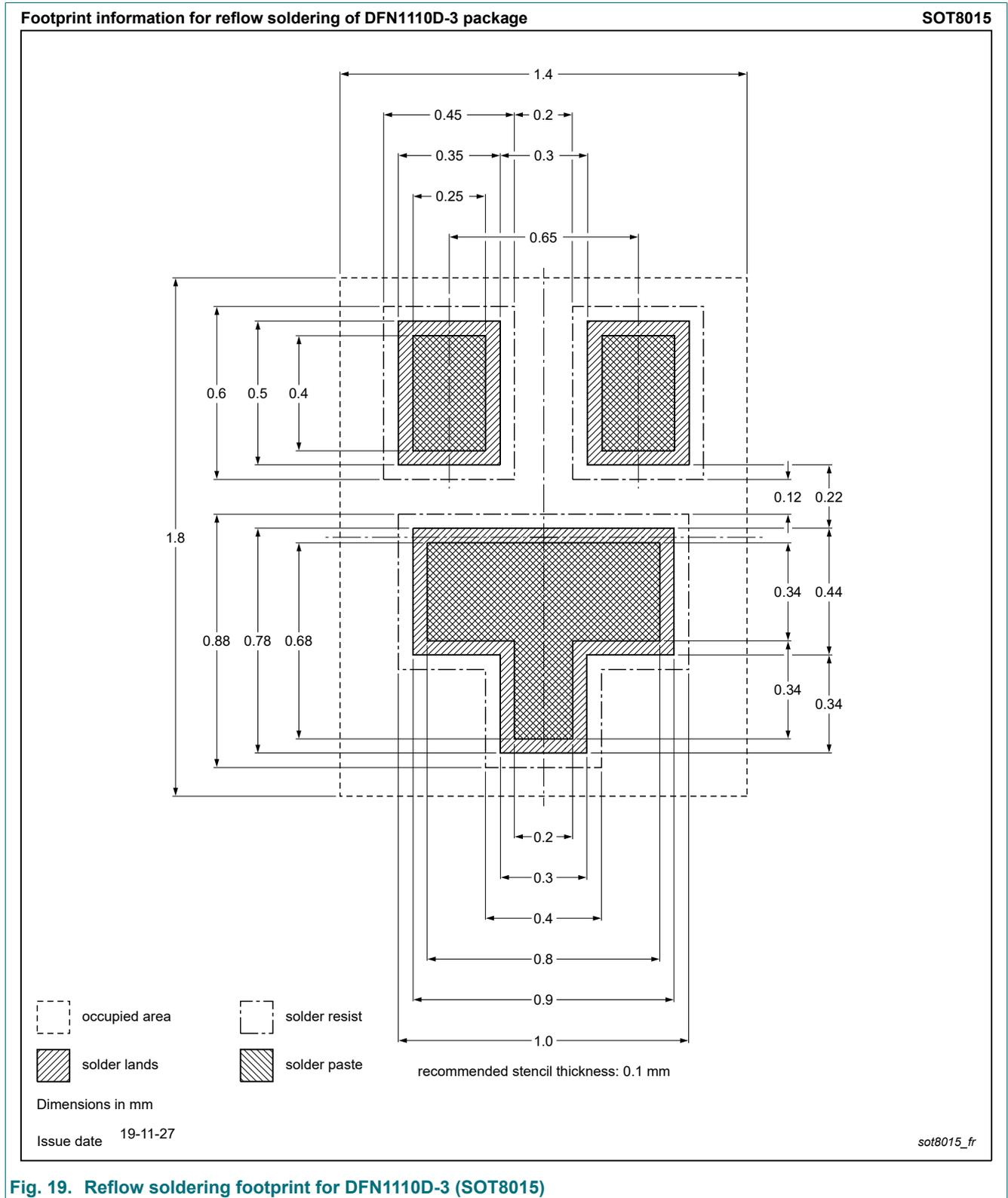
**Fig. 19. Reflow soldering footprint for DFN1110D-3 (SOT8015)**
