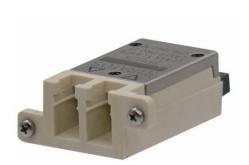
The FNF-LT11 multimode glass optical fiber transceivers provide low profile, cost effective solutions for Fast Ethernet multimode (up to 2.0 km) optical fiber data links with a duplex LC connector interface. These transceivers are fully compliant with the IEEE 802.3u Fast Ethernet standard but can be used for any other data communications purpose within their operating parameters.
