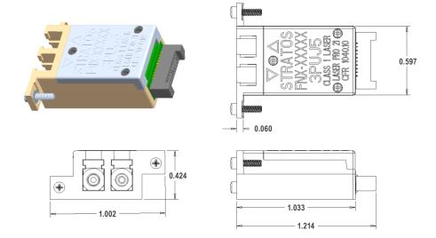
All dimensions in inches. All dimensions +- 0.005", unless noted Screw torque 0.50 +/- 0.10 in-lbs
