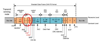
Figure 4 Transmitter - winning CAN FD node
