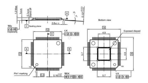
Figure 13 Package Outlines TQFP-100 for TC23x
