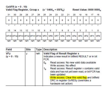
Figure 7 Register GxVFR in the VADC Module of TC2xx Devices
