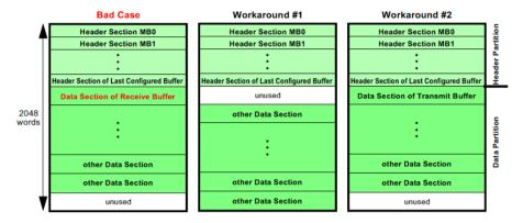
Figure 3 Message RAM Configurations
