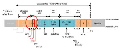
Figure 6 Now receiver (same node as previous figure) - loosing CAN FD node
