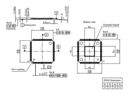
Figure 12 Package Outlines TQFP-144 for TC23x
