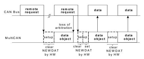
Figure 9 Loss of Arbitration
