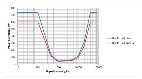
Figure 14 Ripple Voltage vs. Frequency Characteristic
