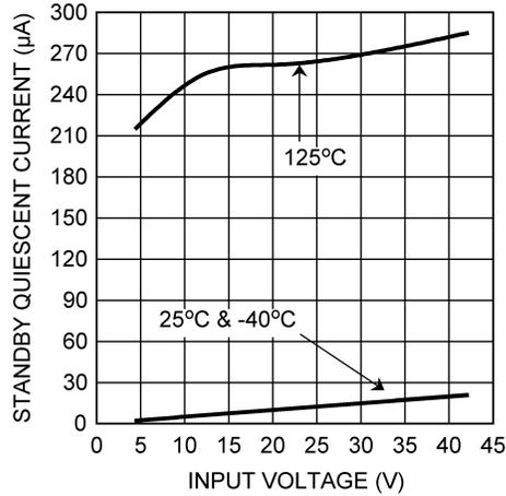
Figure 7. Standby Quiescent Current vs Input Voltage
