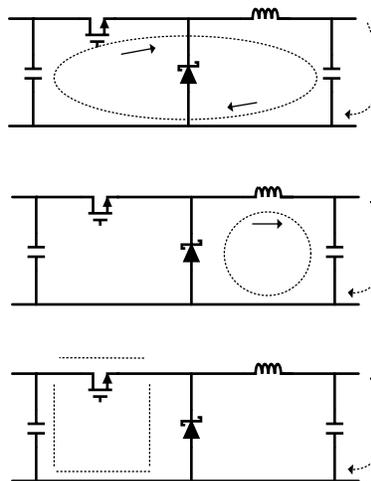
Figure 16. Current Flow in a Buck Application
