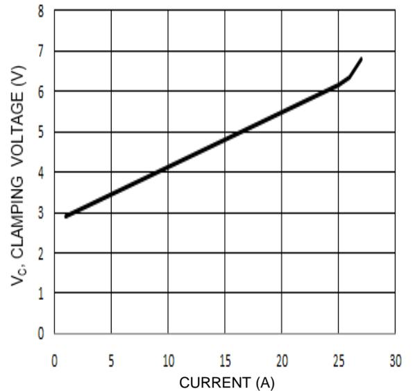
Figure 4 Clamping Voltage Characteristic ( $t_p = 8/20\mu s$ )
