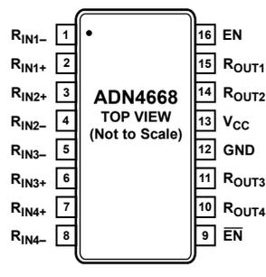
Figure 6. Pin Configuration
