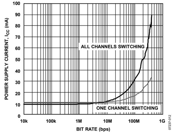
Figure 12. Power Supply Current,  $I_{CC}$  vs. Bit Rate
