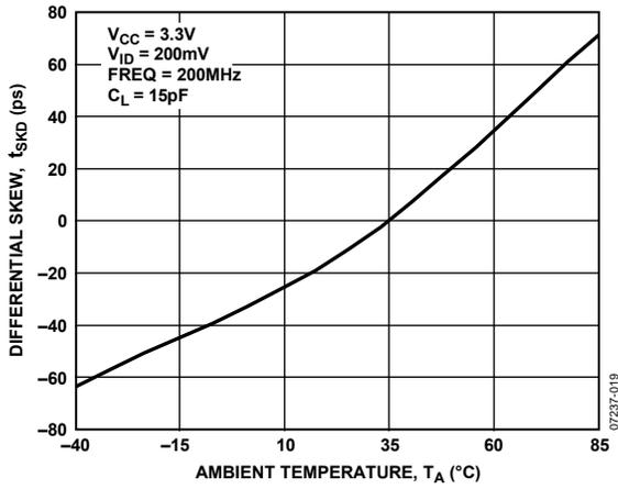
Figure 19. Differential Skew,  $t_{skD}$  vs. Ambient Temperature,  $T_A$
