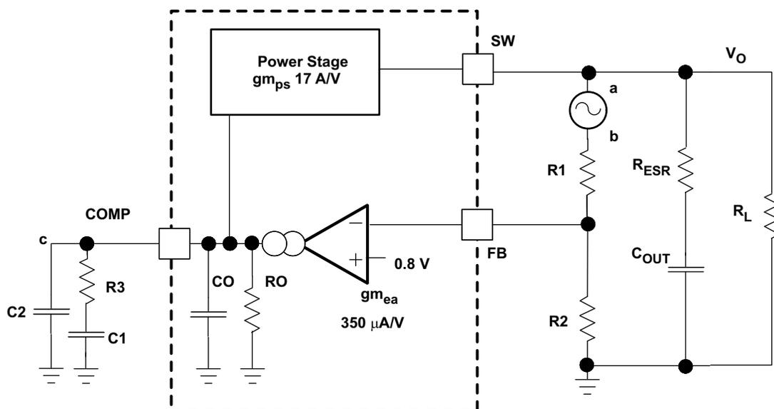
**Figure 30. Small Signal Model for Loop Response**
