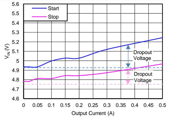
Figure 22. 5 V Start and Stop Voltage (see *Low Dropout Operation and Bootstrap Voltage (BOOT)*)
