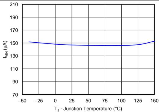
Figure 17.  $V_{IN}$  Supply Current vs Junction Temperature
