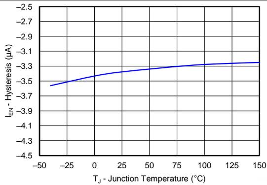
Figure 13. EN Pin Current Hysteresis vs Junction Temperature
