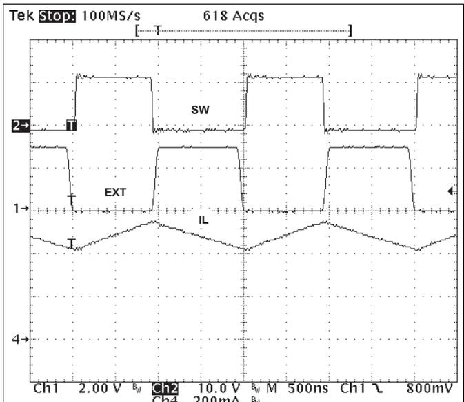
Figure 27. Plot of Synchronizing in CCM
