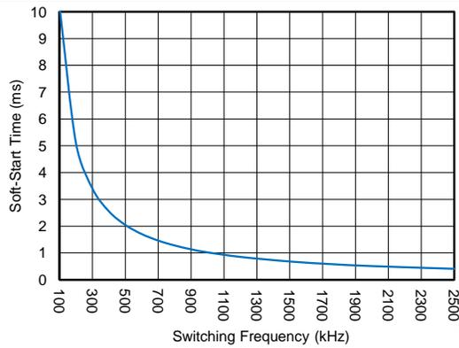
Figure 21. Soft-Start Time vs Switching Frequency
