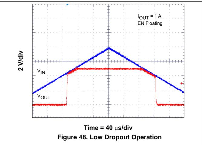
Figure 48. Low Dropout Operation
