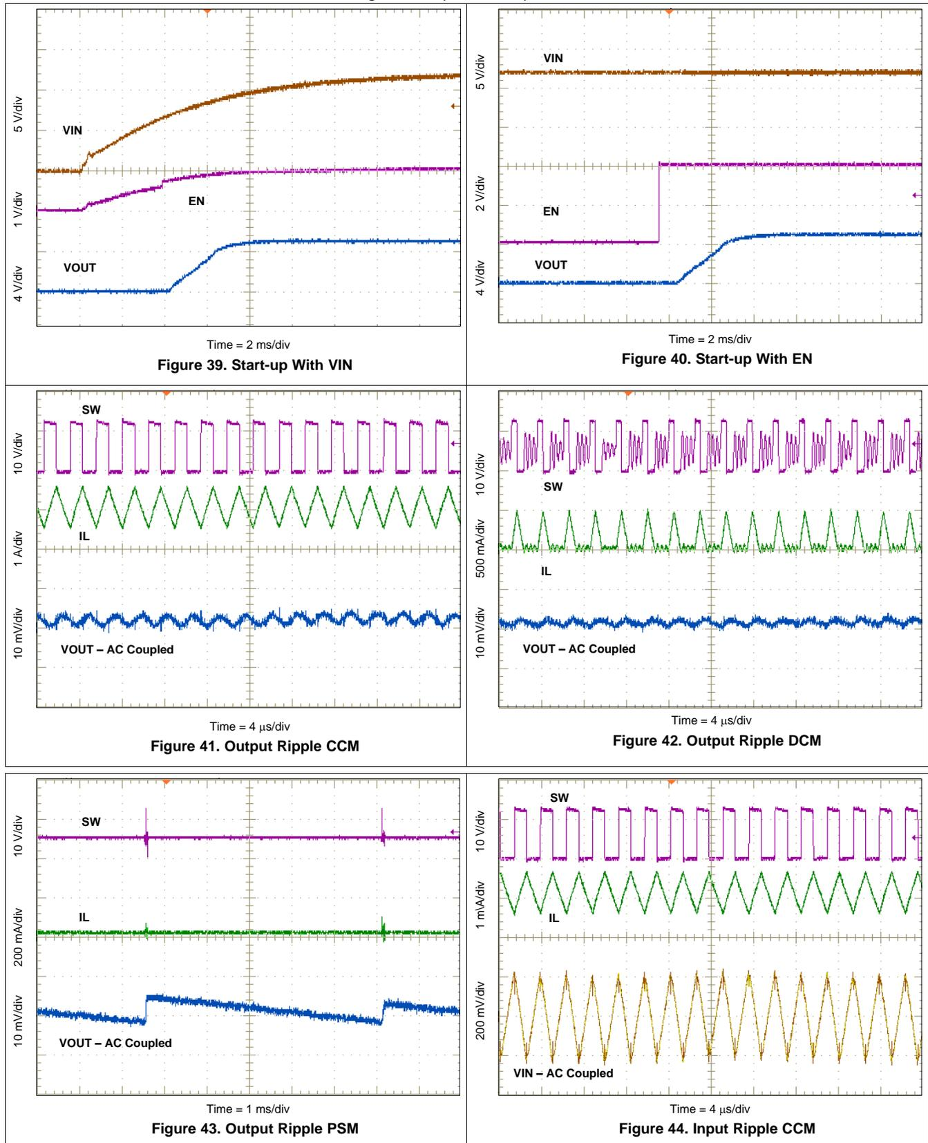
Measurements are taken with standard EVM using a 12V input, 5V output, and 5A load unless otherwise noted.
