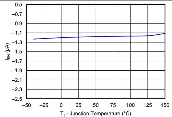
Figure 12. EN Pin Current vs Junction Temperature
