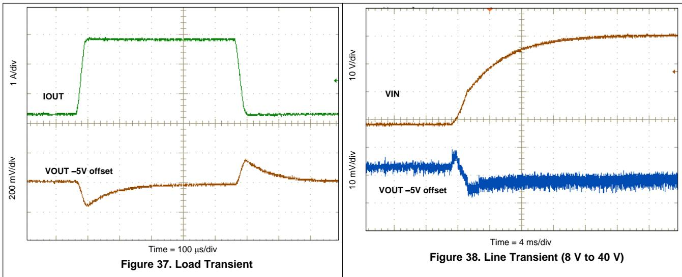
Measurements are taken with standard EVM using a 12V input, 5V output, and 5A load unless otherwise noted.
