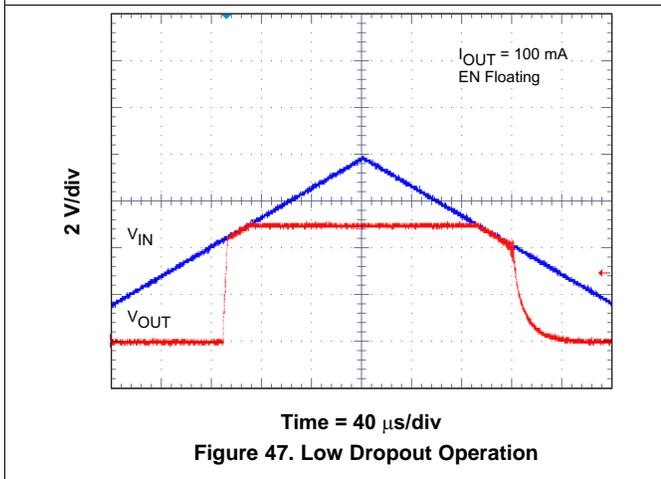
Figure 47. Low Dropout Operation
