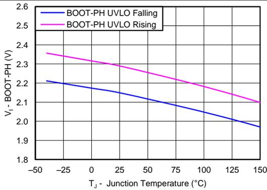
Figure 19. BOOT-SW UVLO vs Junction Temperature
