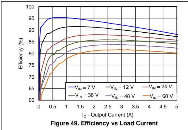
Figure 49. Efficiency vs Load Current
