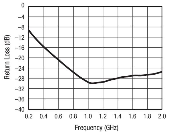
Figure 6. Return Loss in Attenuation State vs Frequency
