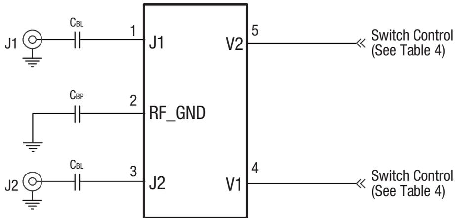
Note:  $C_{BL} = 33 \text{ pF}$ ,  $C_{BP} = 39 \text{ pF}$  for 900 MHz operation.
