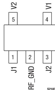
Figure 2. AA116-72LF Pinout – 5-Pin SOT-5 (Top View)
