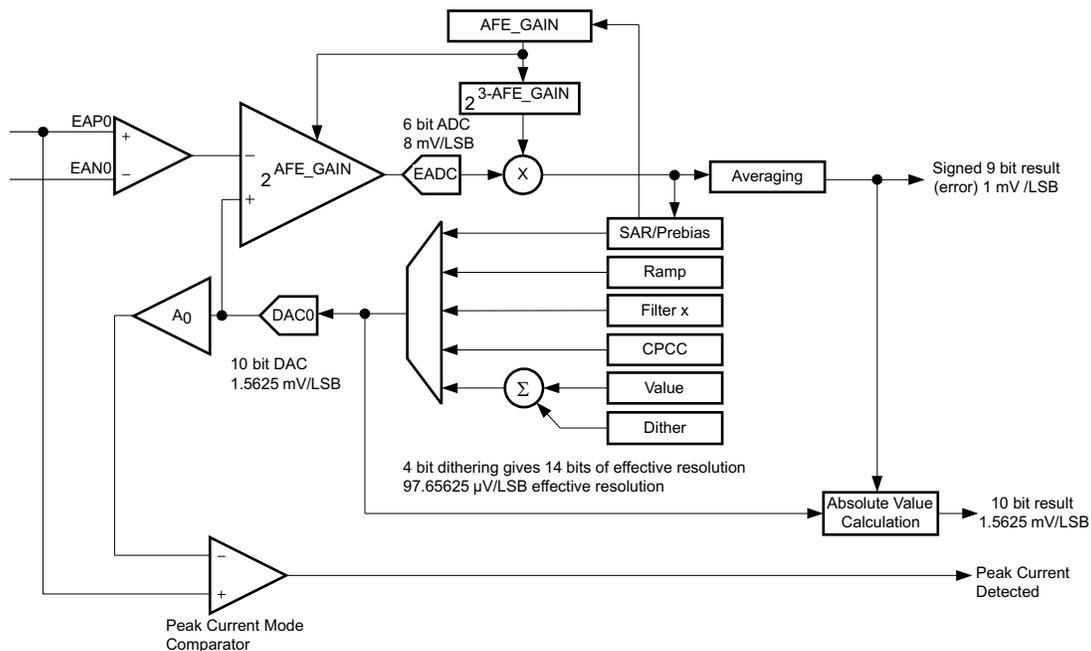
Figure 5-4. Front End Module
