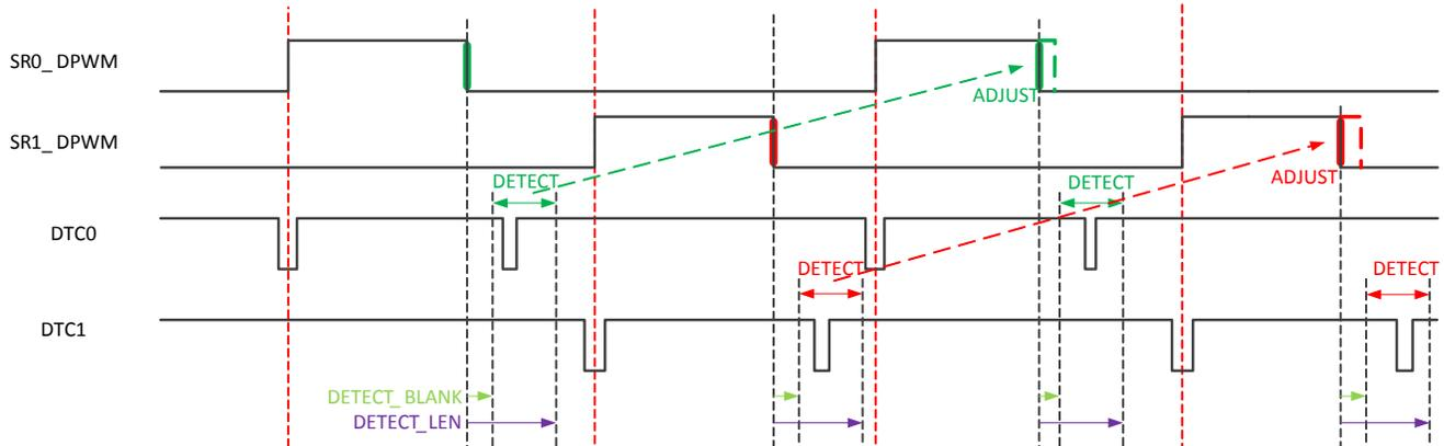
Figure 5-7. Timing Diagram of the DTC Interface
