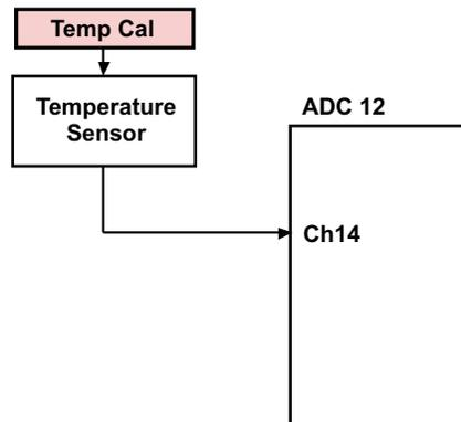
**Figure 7-15. Internal Temp Sensor**
