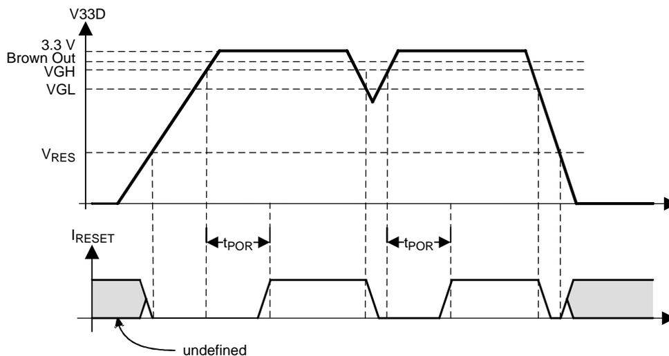
Figure 6-2. Power-On Reset (POR) and Brown-Out Reset (BOR)
