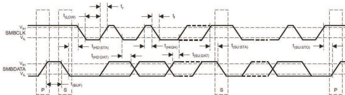
Figure 5-1. I<sup>2</sup>C/SMBus/PMBus Timing Diagram
