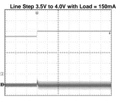
CH2: V<sub>IN</sub>; Scale: 1V/Div, DC Coupled CH3: V<sub>OUT</sub>; Scale: 20mV/Div, AC Coupled
