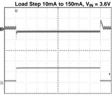
CH3:  $V_{OUT}$ ; Scale: 50mV/Div, AC Coupled CH4:  $I_{OUT}$ ; Scale: 100mA/Div Time scale: 40 $\mu$ s/Div Figure 8.
