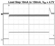
CH3: V<sub>OUT</sub>; Scale: 50mV/Div, AC Coupled CH4: I<sub>OUT</sub>; Scale: 100mA/Div
