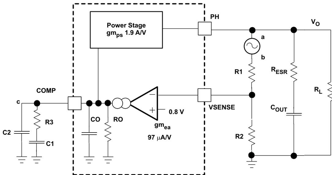
Figure 31. Small Signal Model for Loop Response
