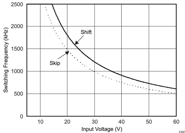
**Figure 45. Maximum Switching Frequency vs Input Voltage**
