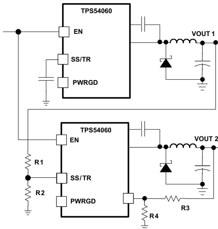
Figure 41. Schematic for Ratiometric and Simultaneous Start-Up Sequence
