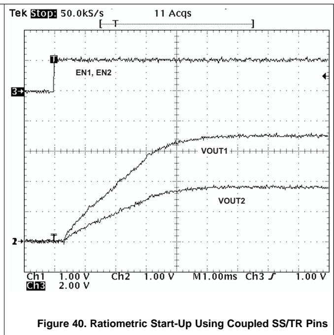
Figure 40. Ratiometric Start-Up Using Coupled SS/TR Pins
