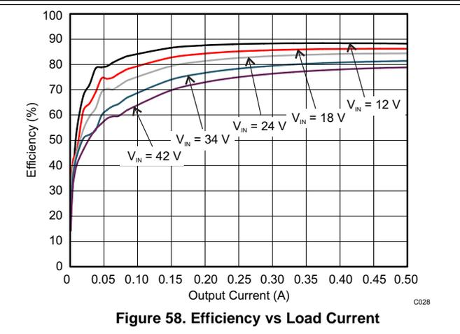
Figure 58. Efficiency vs Load Current
