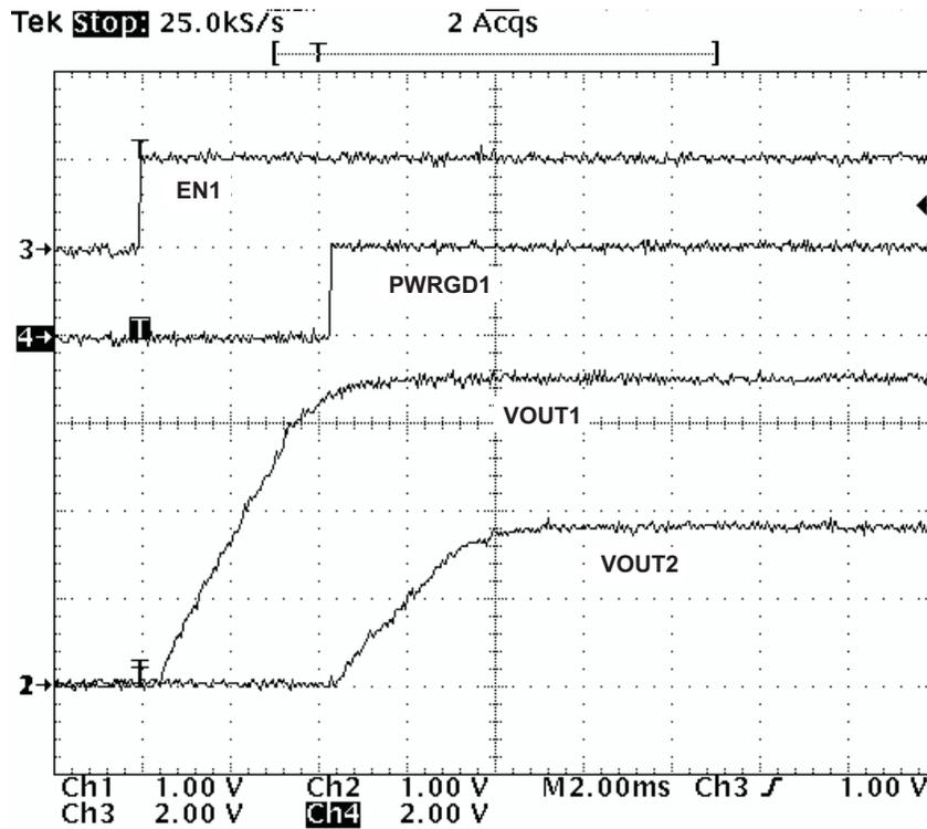
Figure 38. Sequential Startup Using EN and PWRGD
