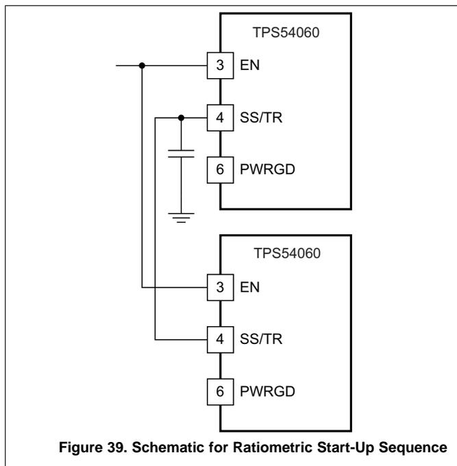
Figure 39. Schematic for Ratiometric Start-Up Sequence
