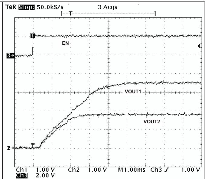
Figure 43. Ratiometric Startup With Tracking Resistors
