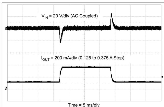
Figure 51. Load Transient
