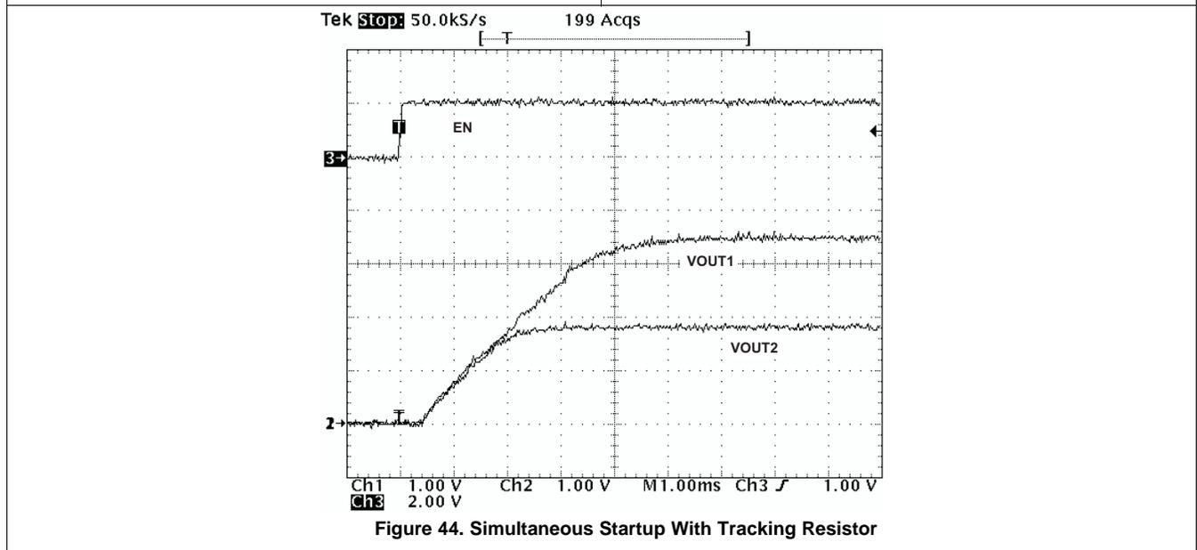
Figure 44. Simultaneous Startup With Tracking Resistor
