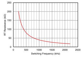
Figure 31. RT vs Frequency Curve
