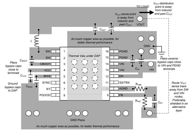
Figure 65. LM43602-Q1 Layout Example
