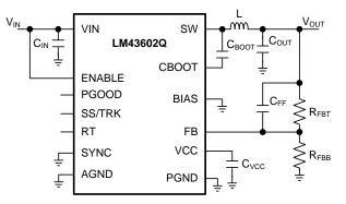
Figure 37. LM43602-Q1 Basic Schematic for V<sub>OUT</sub> < 3.3 V, tie BIAS to Ground
