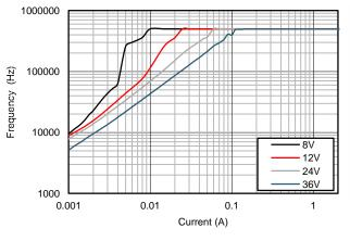
Figure 35.  $V_{OUT} = 5 V F_s = 500 kHz$ Pulse Frequency Mode Operation
