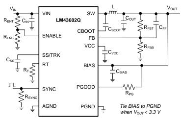
Figure 38. LM43602-Q1 Schematic With All Features
