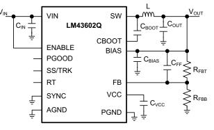
Figure 36. LM43602-Q1 Basic Schematic for  $V_{OUT} \ge 3.3$  V, tie BIAS to  $V_{OUT}$
