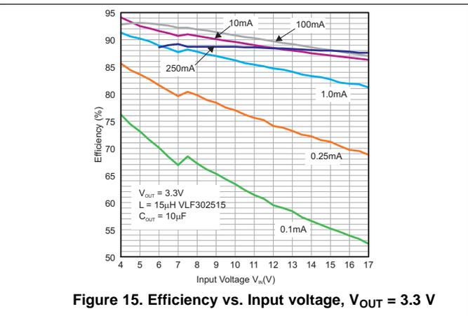
Figure 15. Efficiency vs. Input voltage,  $V_{OUT} = 3.3$  V
