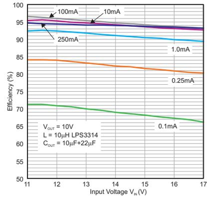
Figure 23. Efficiency vs. Input Voltage,  $V_{OUT} = 10\text{ V}$
