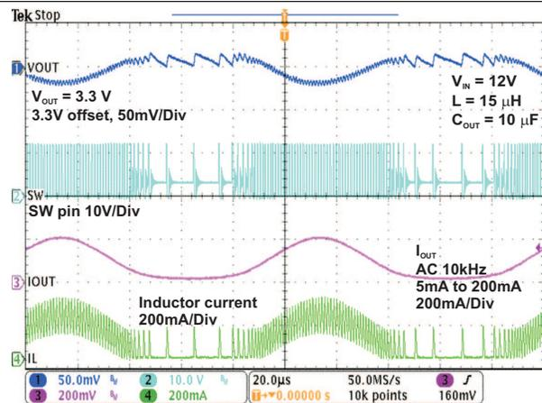
Figure 39. AC Load Regulation,  $V_{OUT} = 3.3\text{ V}$
