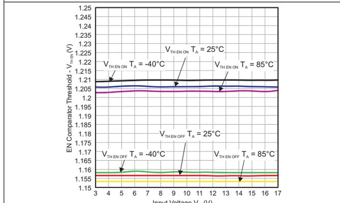
Figure 5. EN Comparator Thresholds vs. Input Voltage
