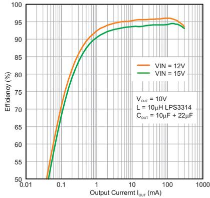
Figure 22. Efficiency vs. Output Current,  $V_{OUT} = 10\text{ V}$
