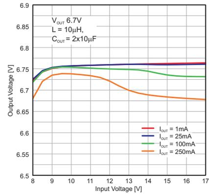
Figure 29. Output voltage vs. Input voltage,  $V_{OUT} = 6.7V$
