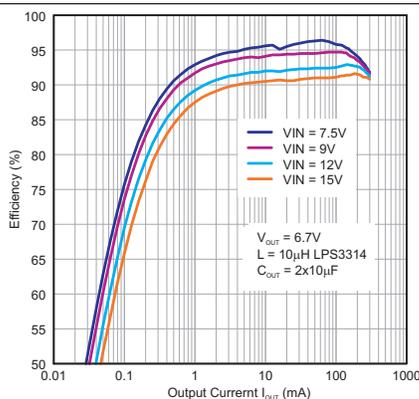
Figure 18. Efficiency vs. Output current,  $V_{OUT} = 6.8\text{ V}$
