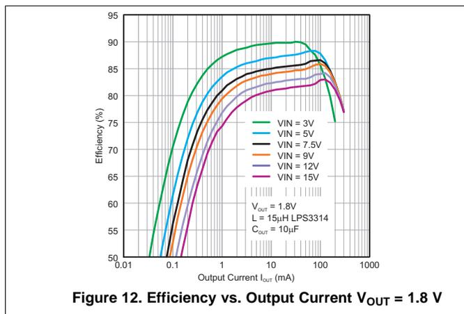
Figure 12. Efficiency vs. Output Current  $V_{OUT} = 1.8$  V
