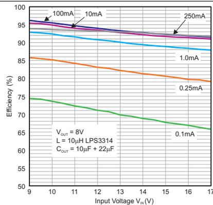
Figure 21. Efficiency vs. Input Voltage,  $V_{OUT} = 8\text{ V}$
