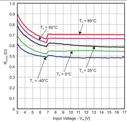
**Figure 7.  $R_{DS(on)}$  Low-Side Switch (Rectifier)**
