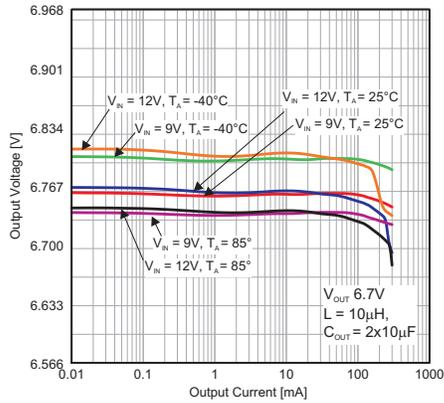
Figure 28. Output Voltage vs. Output Current,  $V_{OUT} = 6.7V$
