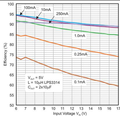
Figure 17. Efficiency vs. Input Voltage,  $V_{OUT} = 5\text{ V}$
