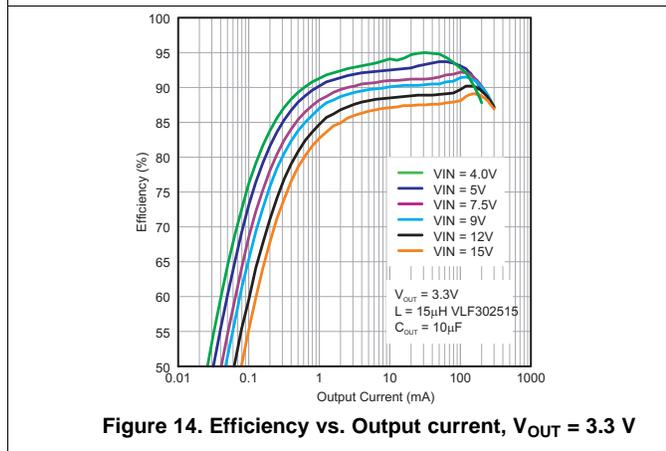
Figure 14. Efficiency vs. Output current,  $V_{OUT} = 3.3$  V
