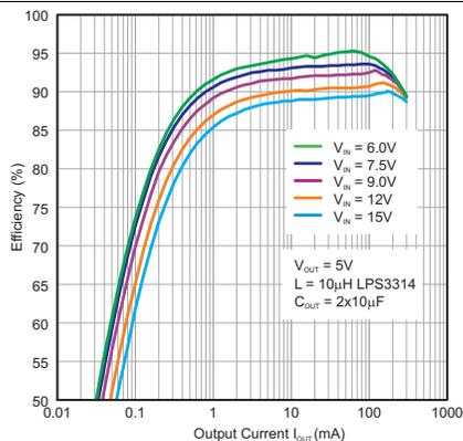
Figure 16. Efficiency vs. Output Current,  $V_{OUT} = 5\text{ V}$
