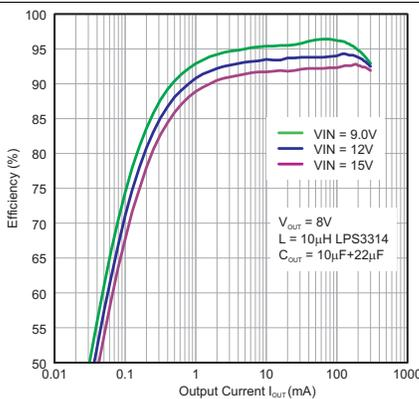
Figure 20. Efficiency vs. Output Current,  $V_{OUT} = 8\text{ V}$
