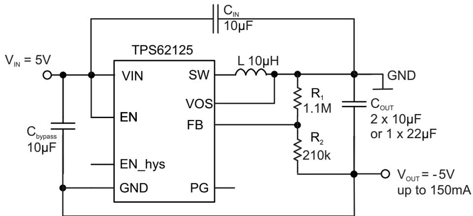
Figure 60. 5 V to -5 V Inverter Configuration, See [SLVA514](#)
