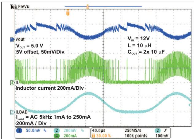
Figure 42. AC Load Regulation  $V_{OUT} = 5\text{ V}$
