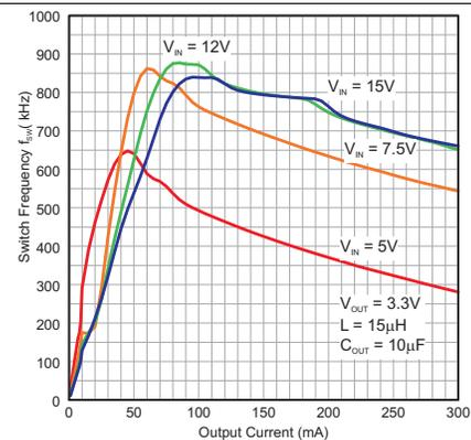
Figure 33. Switch Frequency vs. Output Current,  $V_{OUT} = 3.3V$
