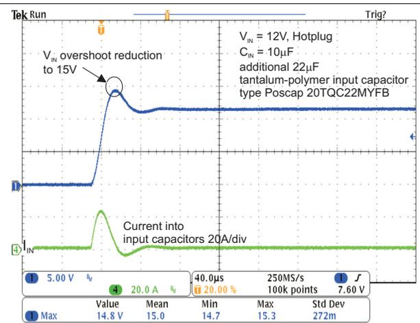
Figure 45.  $V_{IN}$  Hotplug Overshoot Reduction With Poscap
