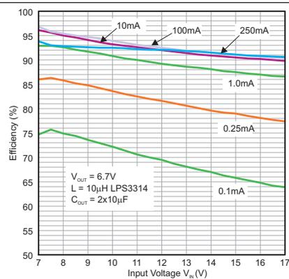
Figure 19. Efficiency vs. Input Voltage,  $V_{OUT} = 6.8\text{ V}$
