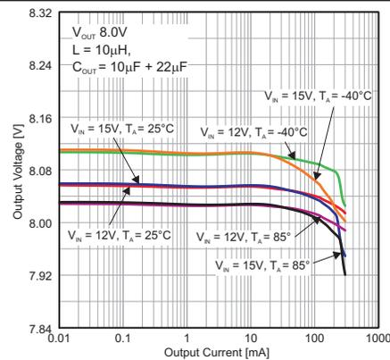
Figure 30. Output Voltage vs. Output Current,  $V_{OUT} = 8V$
