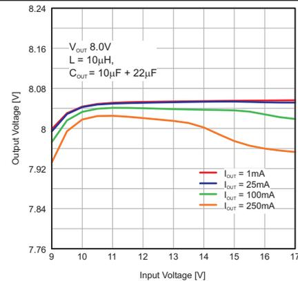
Figure 31. Output Voltage vs. Input Voltage,  $V_{OUT} = 8V$
