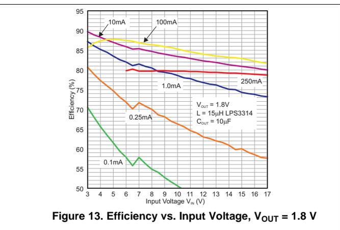
Figure 13. Efficiency vs. Input Voltage,  $V_{OUT} = 1.8$  V
