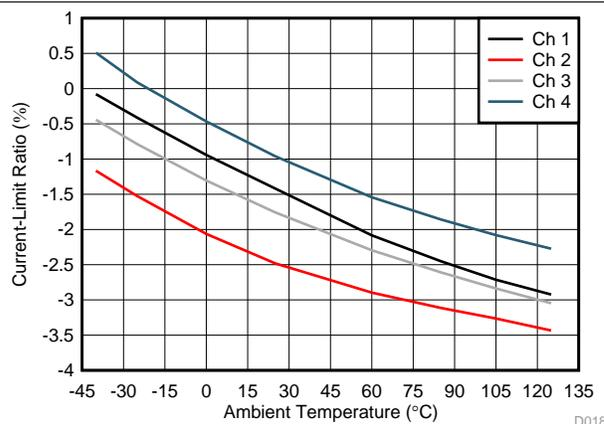
Figure 22. Current-Limit Ratio at 500 mA
