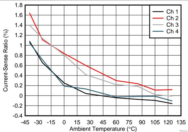
Figure 16. Current-Sense Ratio at 25 mA
