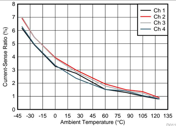
Figure 15. Current-Sense Ratio at 5 mA
