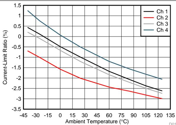
Figure 21. Current-Limit Ratio at 200 mA
