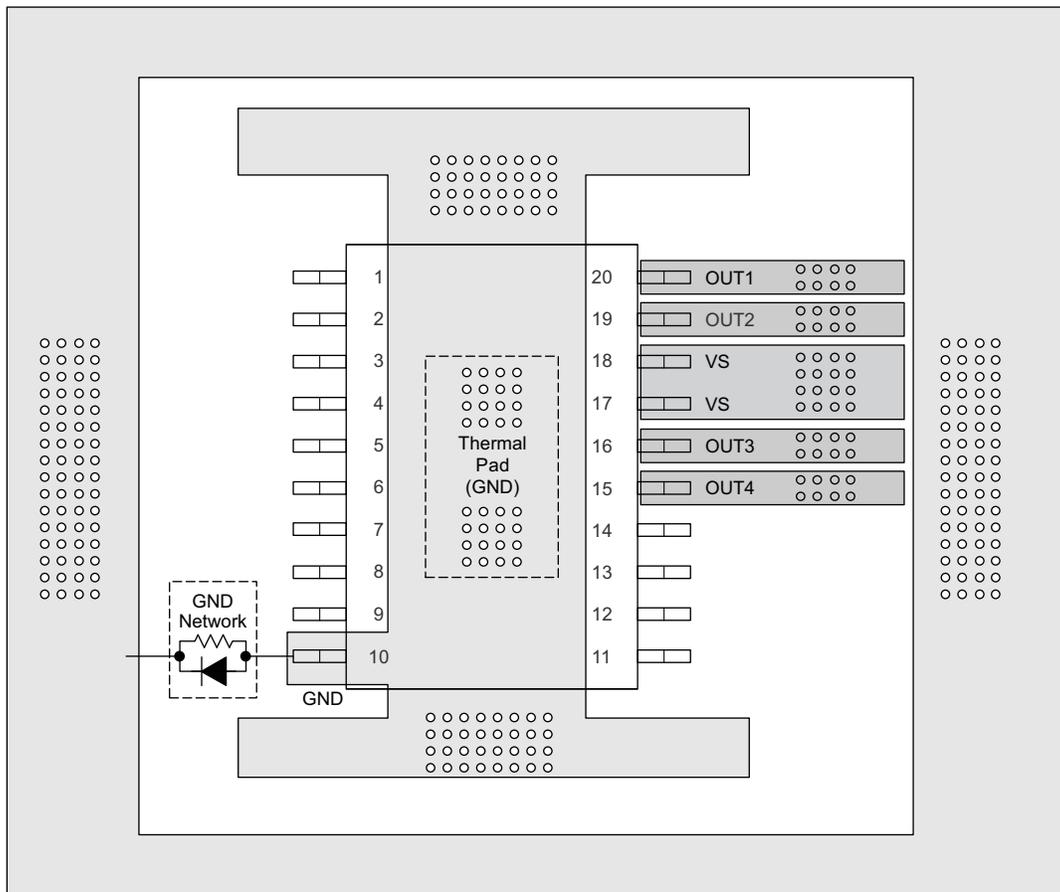
**Figure 44. Layout Example With a GND Network**
