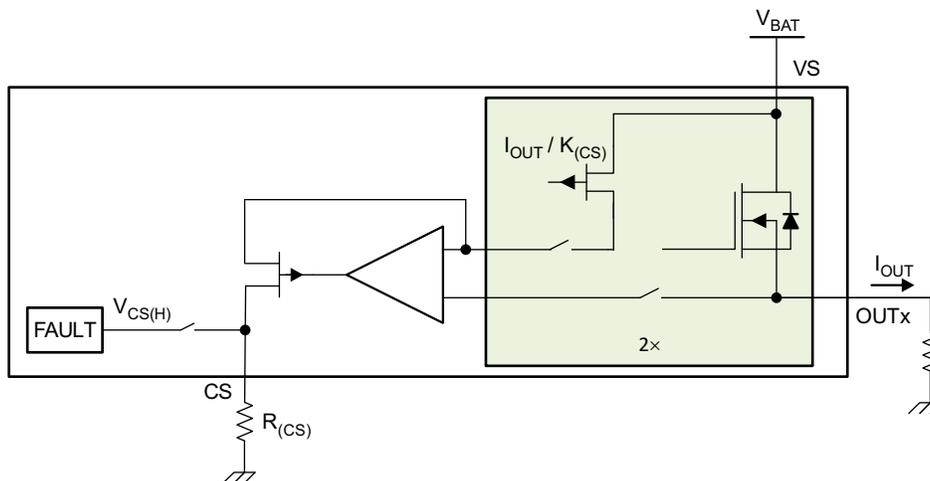
Figure 24. Current-Sense Block Diagram
