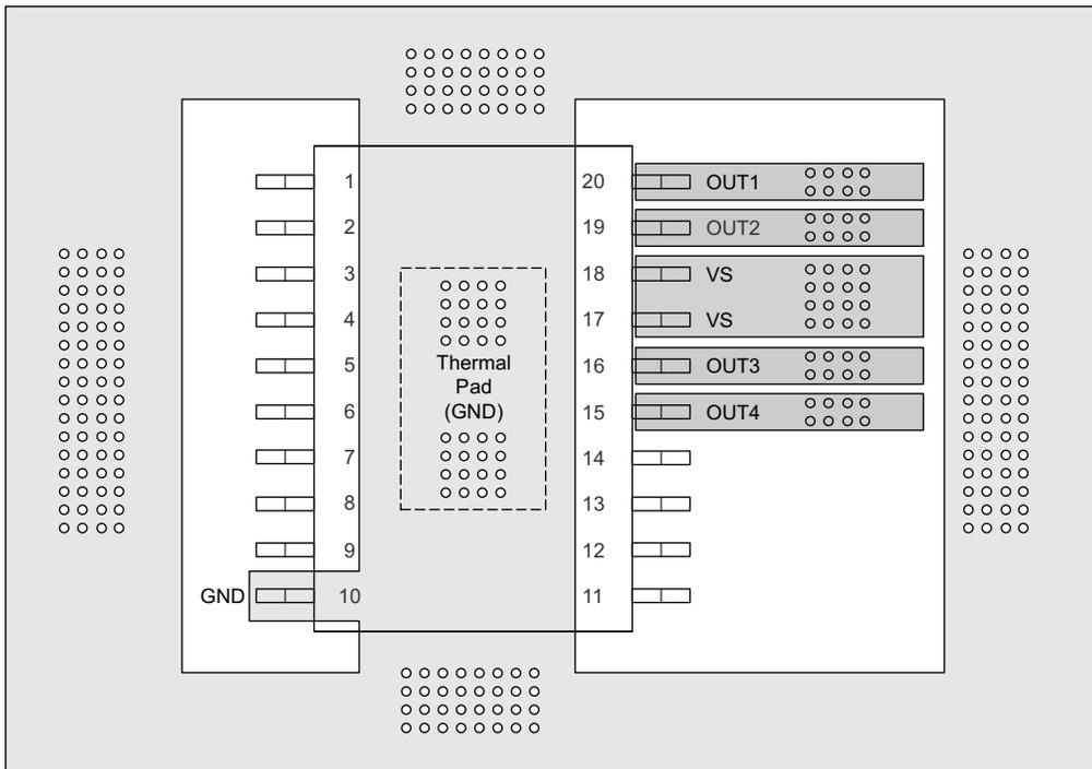
Figure 43. Layout Example Without a GND Network
