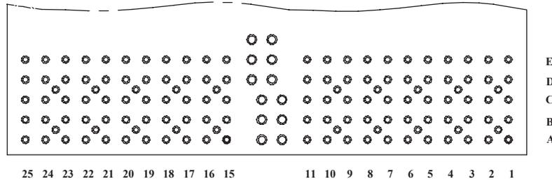
Recommended PCB hole mounting pattern for row differential applications.
