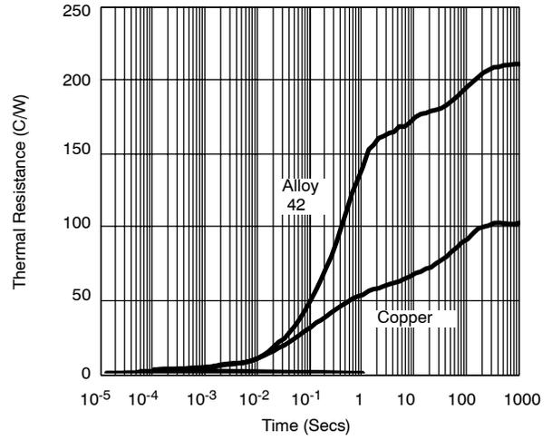
**FIGURE 5.** Leadframe Comparison on Alloy 42 1-inch<sup>2</sup> PCB
