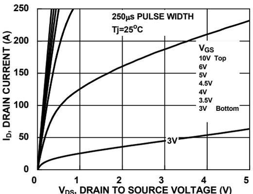
**Figure 9. Saturation Characteristics**
