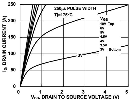
**Figure 10. Saturation Characteristics**
