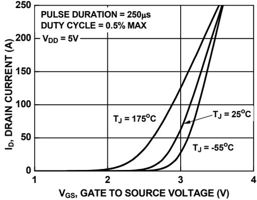
**Figure 7. Transfer Characteristics**
