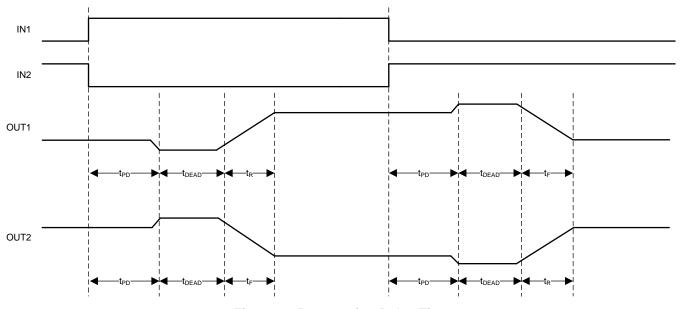
Figure 6. Propagation Delay Time
