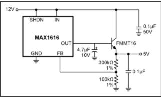
Figure 1. An external emitter-follower increases the output current while maintaining the low quiescent current of this LDO regulator.
