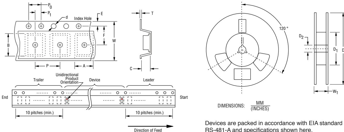
Devices are packed in accordance with EIA standard RS-481-A and specifications shown here.
