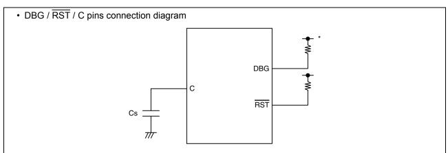
\*: Connect the DBG pin to an external pull-up resistor of 2 k $\Omega$  or above. After power-on, ensure that the DBG pin does not stay at "L" level until the reset output is released. The DBG pin becomes a communication pin in debug mode. Since the actual pull-up resistance depends on the tool used and the interconnection length, refer to the tool document when selecting a pull-up resistor.
