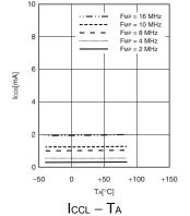
$V_{CC} = 5.5 \text{ V}$ ,  $F_{MPL} = 16 \text{ kHz}$  (divided by 2) Subclock mode with the external clock operating
