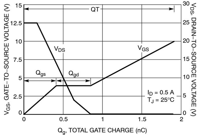
**Figure 6. Gate-to-Source and Drain-to-Source Voltage vs. Total Charge**
