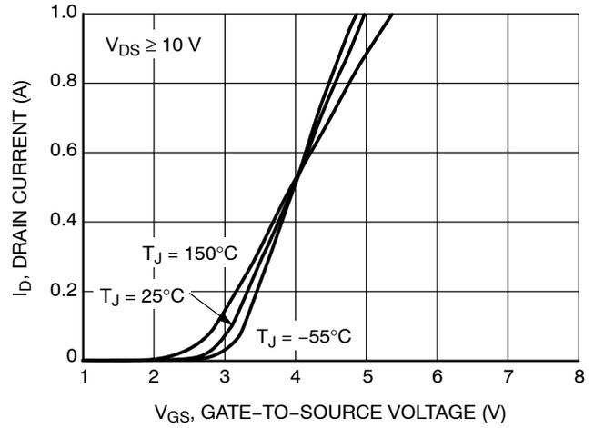
**Figure 4. Transfer Characteristics**
