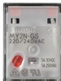
Relay with AC Coil (LED: Red)
