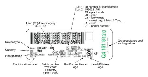
Fig. 5 - 2D Bar Code Label (according the bar code standard for 2D label PDF 417) for a Lead (Pb)-Free Device Made in Philippines, Detailed Description
