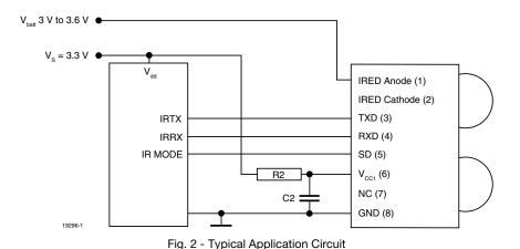
Figure 2 shows an example of a typical application for to work with a separate supply voltage  $V_S$  and using the transceiver with the IRED Anode connected to the unregulated battery  $V_{batt}$ . This method reduces the peak load of the regulated power supply and saves therefore
