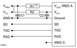
Fig. 1 - Recommended Application Circuit
