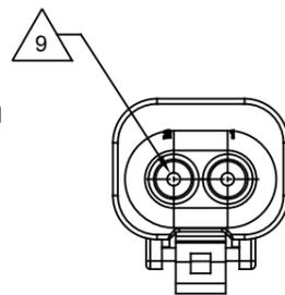
LASER ENGRAVE POLARITY, CONTACT NUMBER, VOLTAGE, SEAL TYPE, SPECIAL CIRCUIT TYPE (RVPC), AND LED COLOR CODE AS SHOWN IN THIS AREA.
