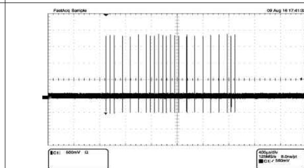
Figure 7-21. Auto-Negotiation Fast Link Pulses Waveform
