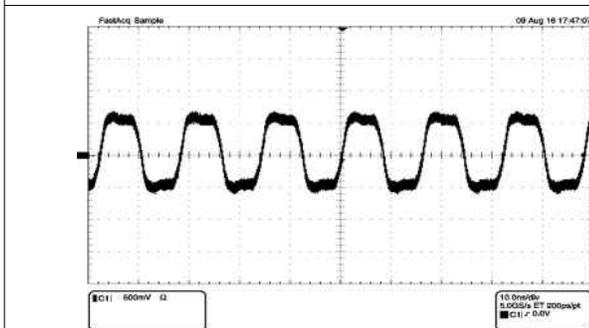
Figure 7-20. 100BASE-FX Waveform
