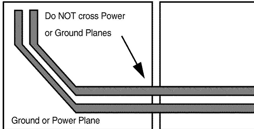
Figure 11-2. Differential Signal Pair and Plane Crossing
