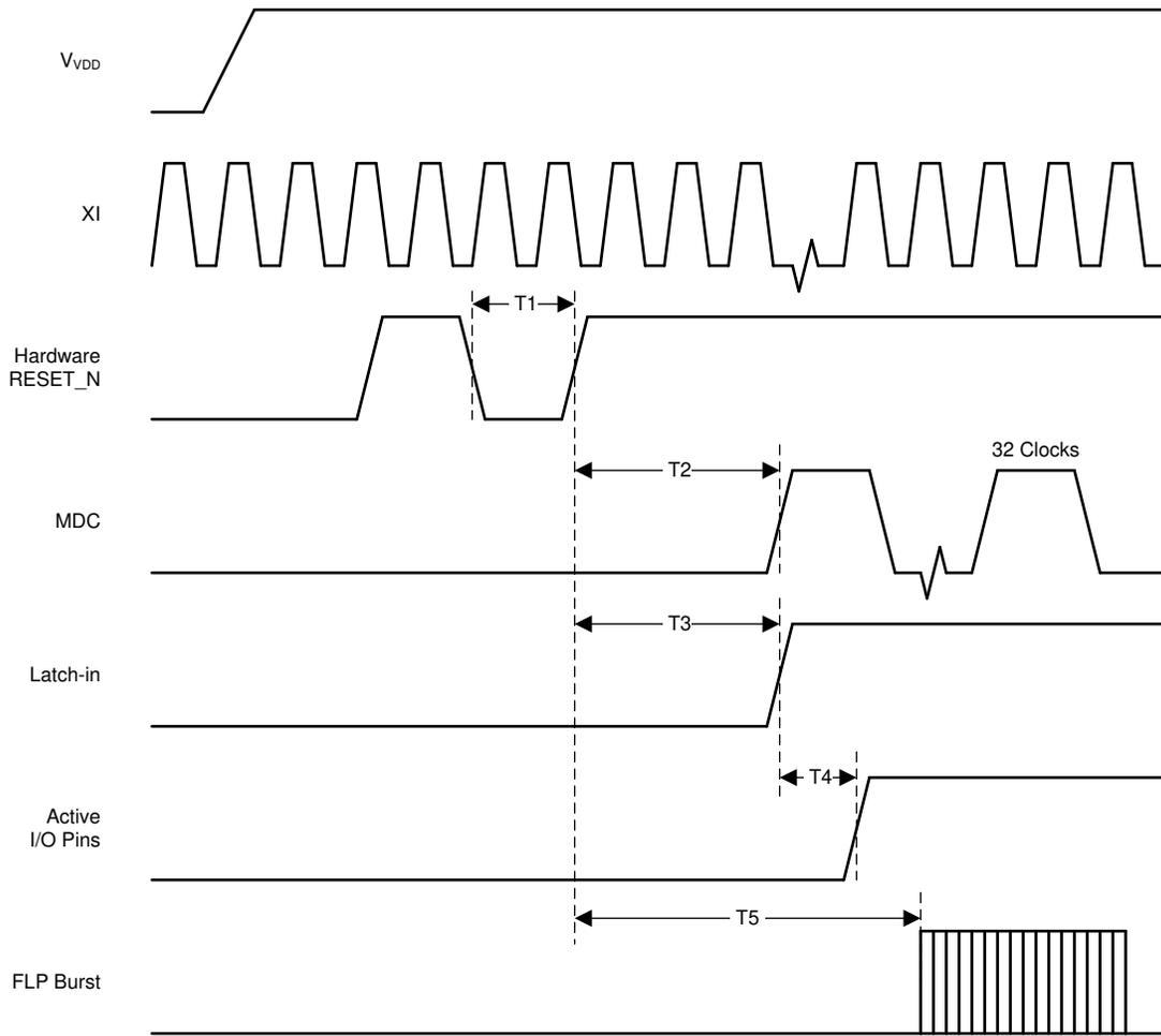
**Figure 7-3. Reset Timing**
