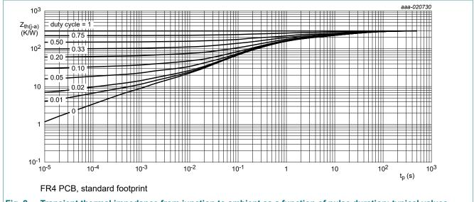
Transient thermal impedance from junction to ambient as a function of pulse duration; typical values
