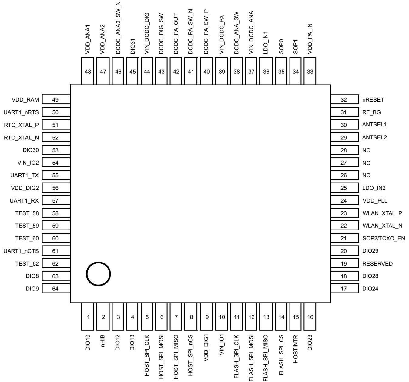
Figure 7-1. Top View Pin Assignment for 64-Pin VQFN
