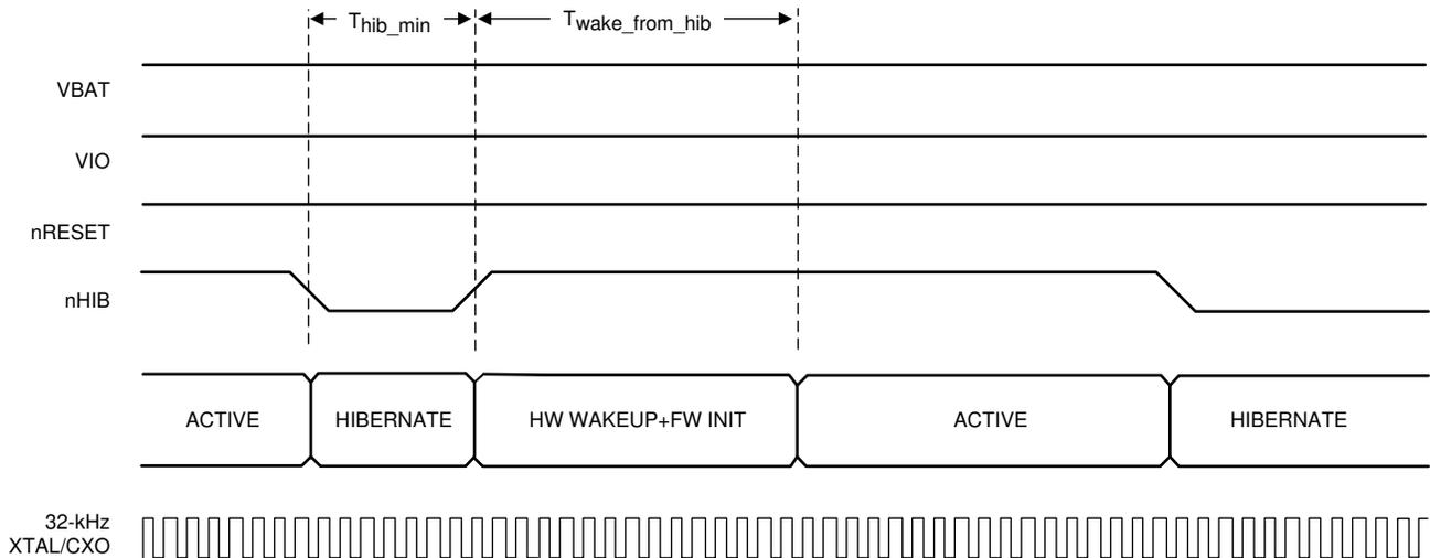
Figure 8-8. nHIB Timing Diagram
