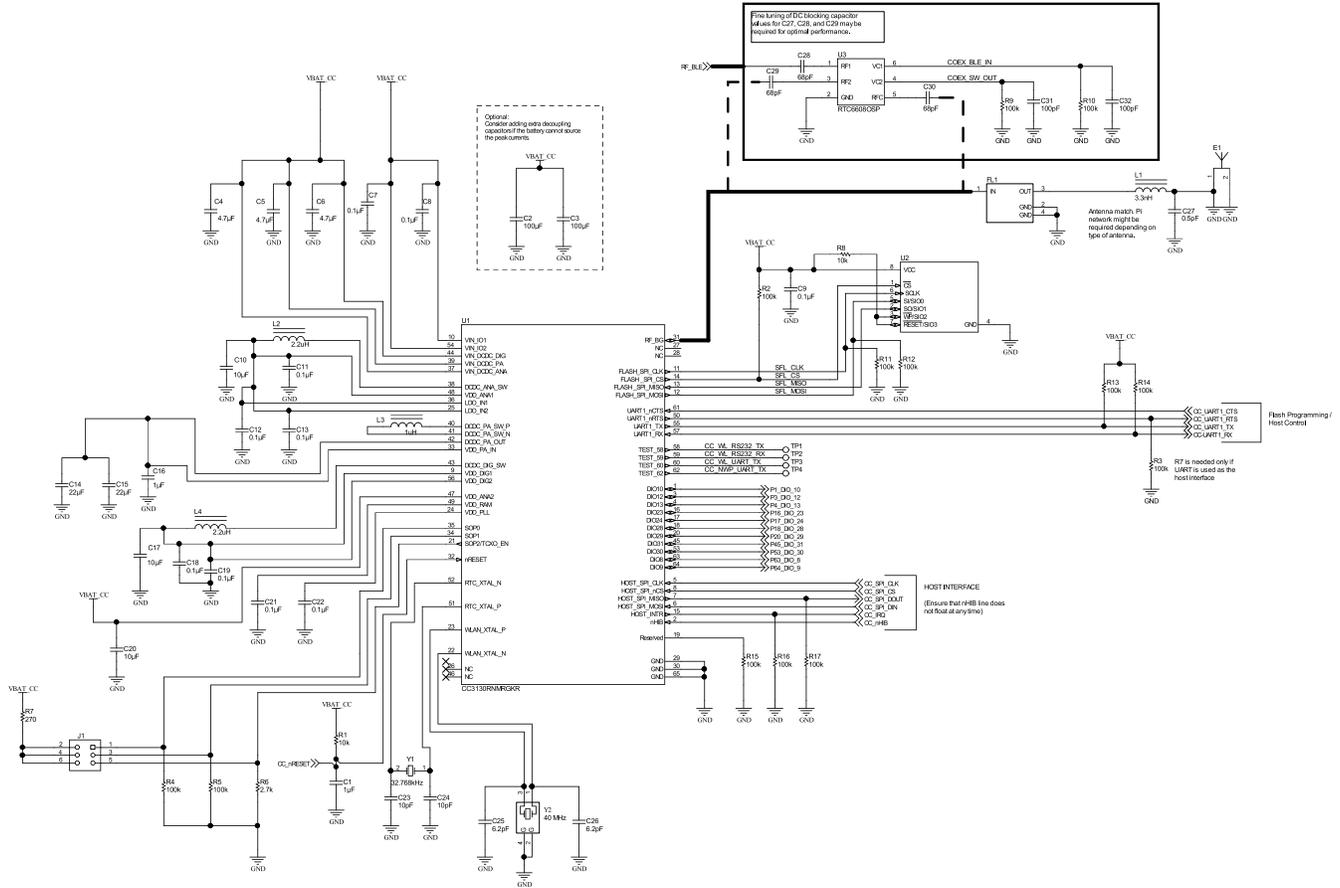
Figure 10-5. CC3130 Engine Area and Optional BLE Coexistence
