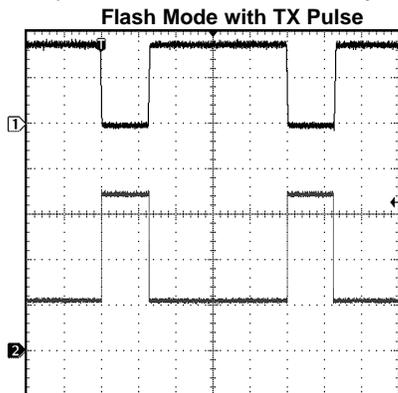
$V_{IN} = 3.6\text{V}$ , Load = 700mA (Flash), LED = PWF1
