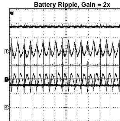
$V_{IN}$  = Li-Ion Battery at 3.7V, Load = 400mA; LED = PWF1;
