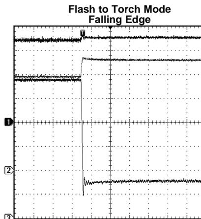
$V_{IN} = 3.6\text{V}$ , Load = 800mA/200mA (Flash/Torch), LED = PWF1
