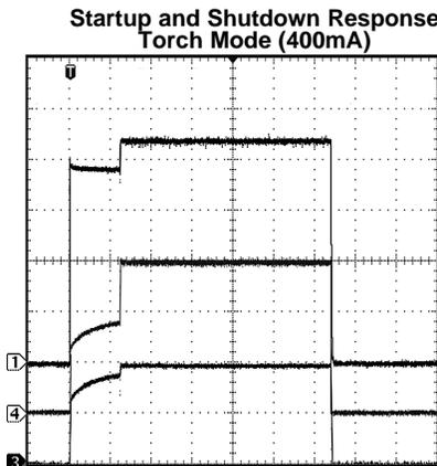
$V_{IN} = 3.6\text{V}$ , Load = 400mA, LED = PWF1;
