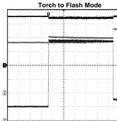
$V_{IN} = 3.6\text{V}$ , Load = 200mA/800mA (Torch/Flash), LED = PWF1;
