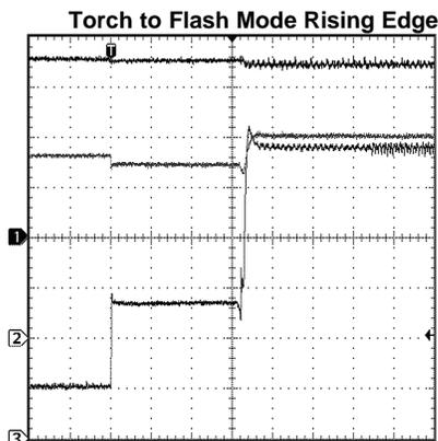
$V_{IN} = 3.6\text{V}$ , Load = 200mA/800mA (Torch/Flash), LED = PWF1
