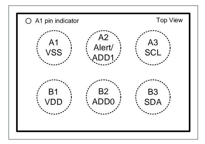
In Figure 3 the pin assignment of the WLCSP package is shown. The viewing side is from the top. The A1 pin is also marked with a point on the top side.
