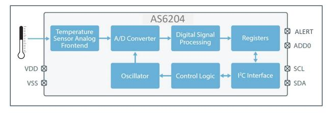
In Figure 2 the functional blocks are depicted. The sensing element for sensing the temperature is a Si bipolar transistor. The analog signal of the sensing element is converted into a digital signal by the A/D converter and the signal is further processed by a digital signal processor and written into the registers. The registers can be accessed via the serial bus interface (I<sup>2</sup>C bus).
