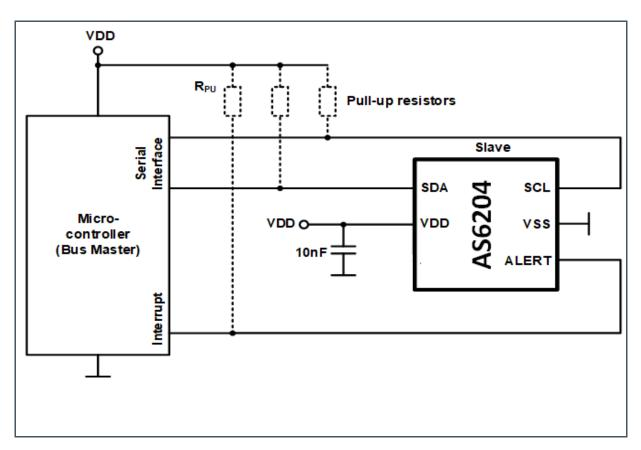
In Figure 33 the connections of the AS6204 temperature sensors to a microcontroller and the supply voltage are shown.
