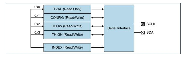
In Figure 8 the registers that the device contains are shown.
