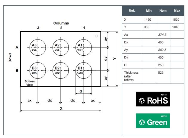
(1) All dimensions are in micrometers. Angles in degrees.
