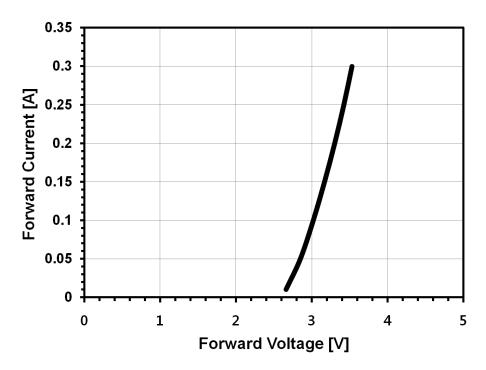
Fig 3. Forward Current vs. Forward Voltage,  $T_a=25^{\circ}C$
