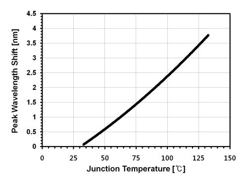
Fig 7. Junction Temperature vs. Peak Wavelength Shift,  $I_F=150mA$
