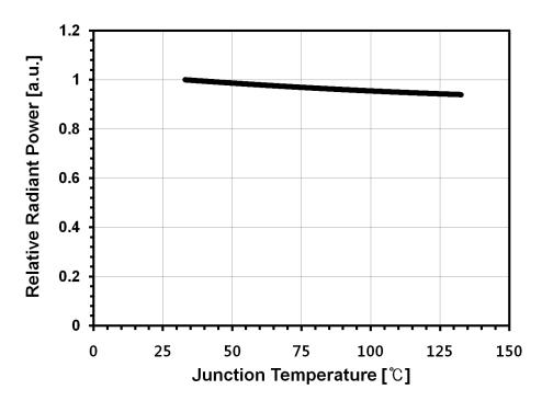
Fig 5. Junction Temperature vs. Relative Radiant Power,  $I_F=150mA$
