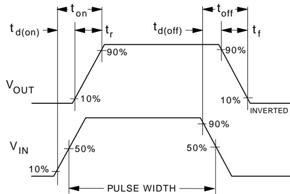
**Figure 12. Switching Waveforms.**
