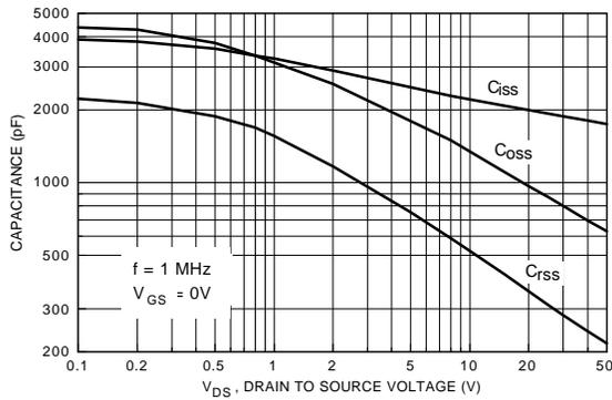
**Figure 9. Capacitance Characteristics.**
