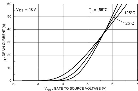
Figure 5. Transfer Characteristics.
