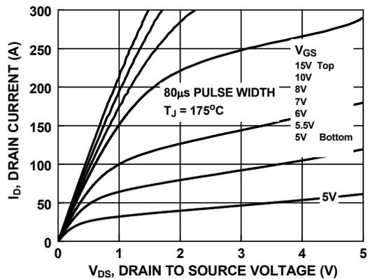
Figure 10. Saturation Characteristics
