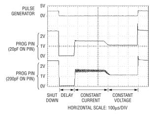
Figure 5. Stability Waveforms
