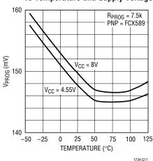
Program Pin Voltage for I<sub>BAT2</sub>/10 vs Temperature and Supply Voltage
