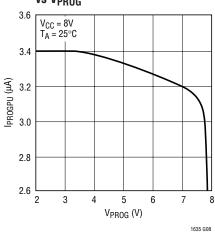
Program Pin Voltage vs Charge Current (50mA)
