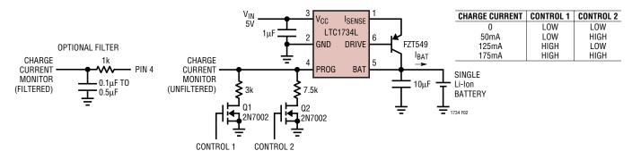
Figure 2. Logic Control Programming of Output Current to OmA, 50mA, 125mA or 175mA
