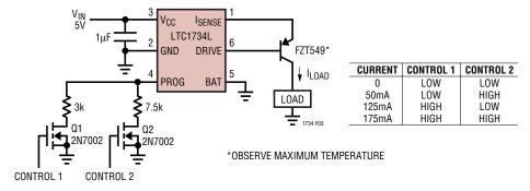
Figure 3. Programmable Current Source with Output Current of OmA, 50mA, 125mA or 175mA
