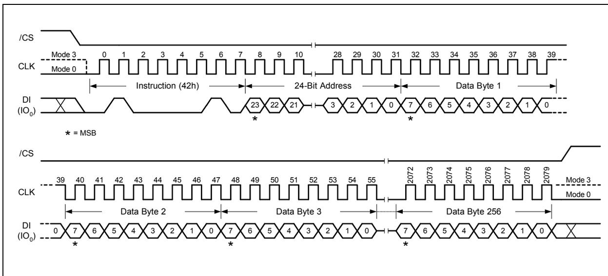
Figure 36. Program Security Registers Instruction (SPI Mode only)
