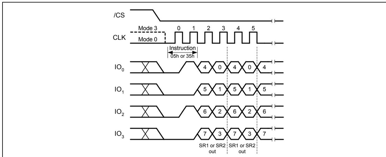
Figure 8b. Read Status Register Instruction (QPI Mode)
