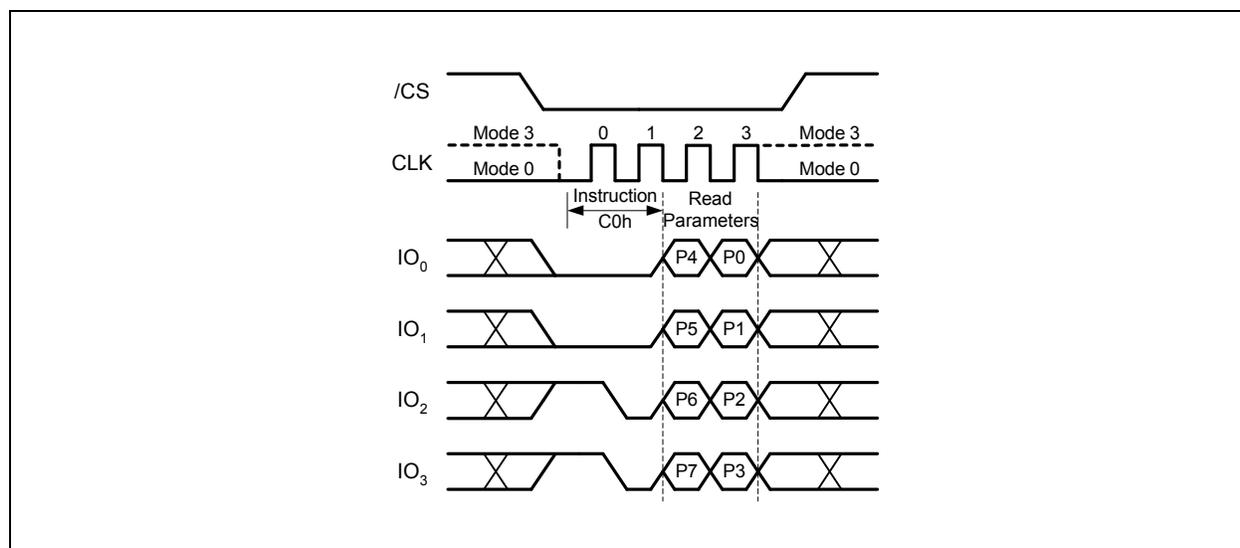
Figure 38. Set Read Parameters Instruction (QPI Mode only)
