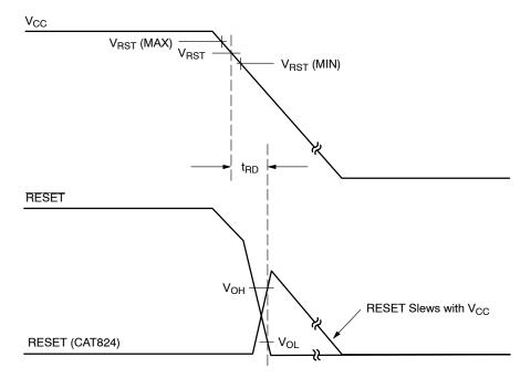
Figure 9. Timing Diagram – Power Down
