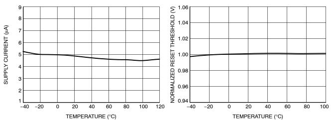
Figure 2. V<sub>CC</sub> Supply Current vs. Temperature
