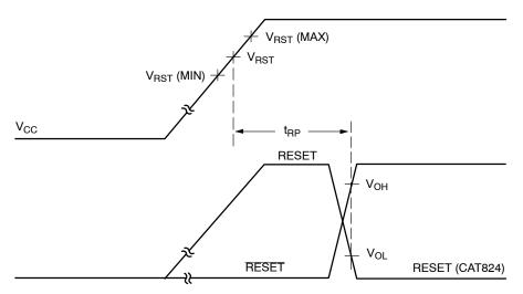
Figure 10. Timing Diagram – Power Up
