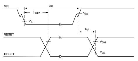
Figure 5. Timing Diagram – Pushbutton RESET
