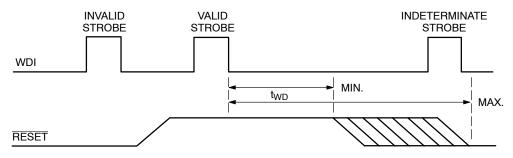
Figure 8. Timing Diagram - Strobe Input
