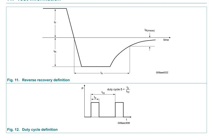
The current ratings for the typical waveforms are calculated according to the equations:  $I_{F(AV)} = I_M \times \delta$  with  $I_M$  defined as peak current,  $I_{RMS} = I_{F(AV)}$  at DC, and  $I_{RMS} = I_M \times \sqrt{\delta}$  with  $I_{RMS}$  defined as RMS current.
