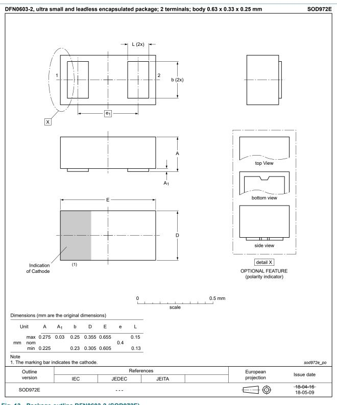
Fig. 13. Package outline DFN0603-2 (SOD972E)
