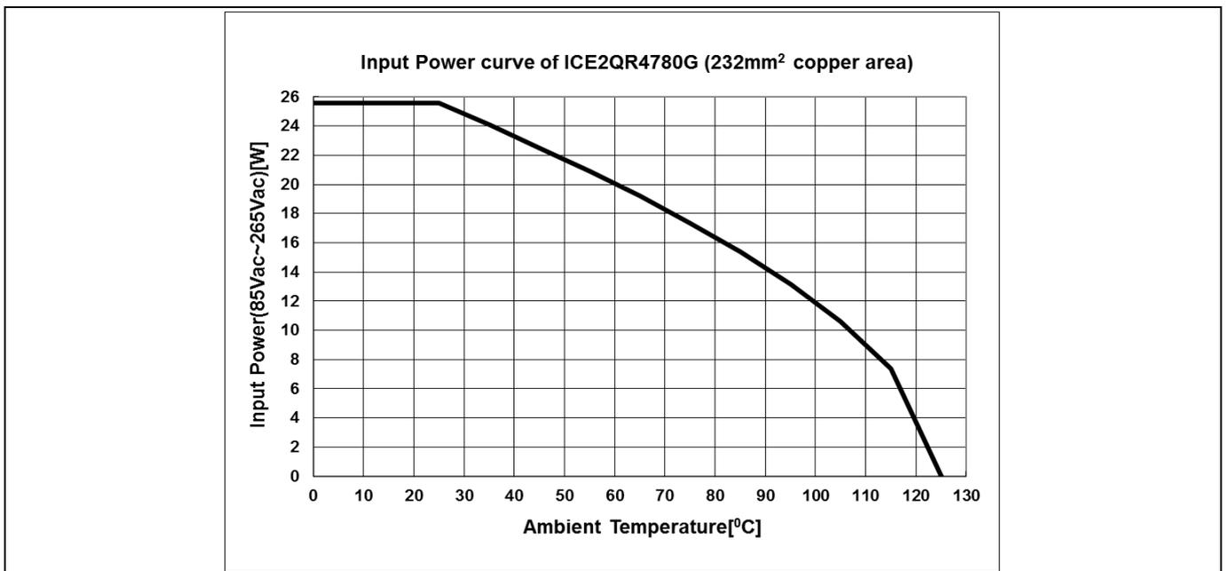
Figure 13 Input power curve  $V_{IN}=85 \sim 265 V_{AC}$ ;  $P_{in}=f(T_a)$
