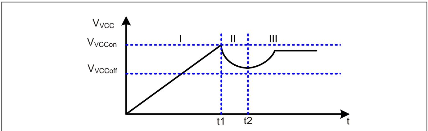
Figure 4 VCC voltage at start up
