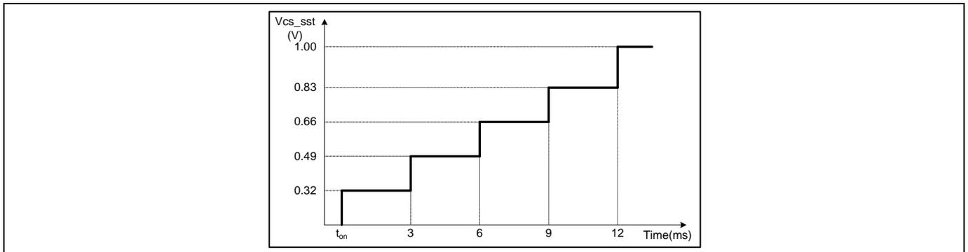
Figure 5 Maximum current sense voltage during soft start
