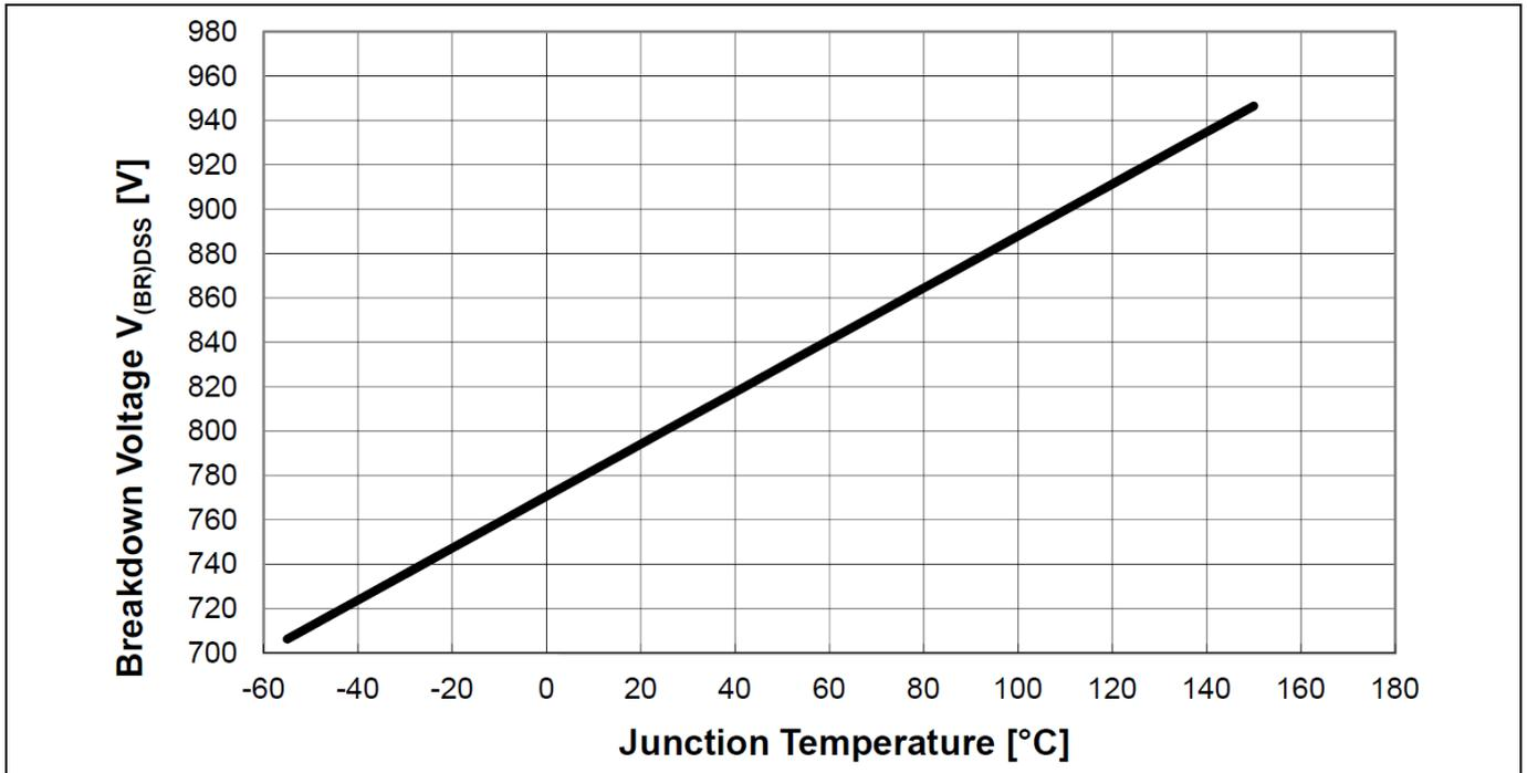
Figure 12 Drain-source breakdown voltage;  $V_{BR(DSS)} = f(T_j)$ ,  $I_D = 0.25mA$
