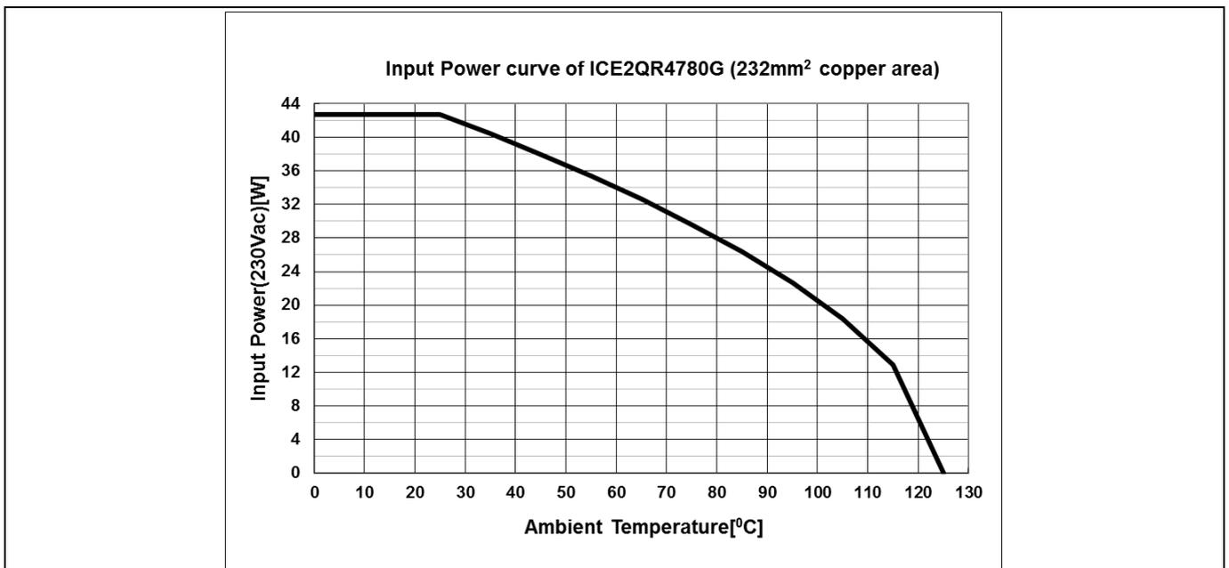
Figure 14 Input power curve  $V_{IN}=230 V_{AC}$ ;  $P_{in}=f(T_a)$
