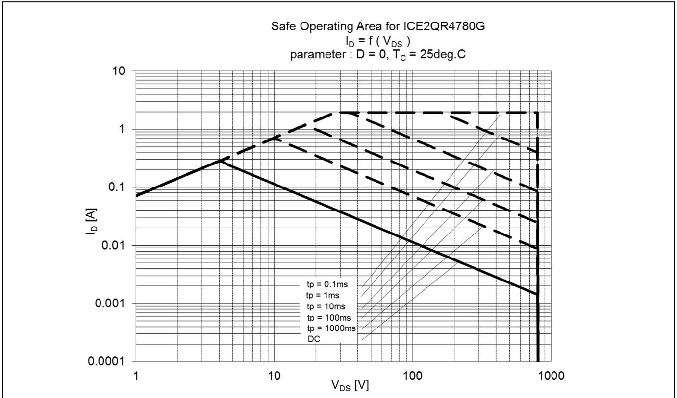
Figure 10 Safe Operating Area (SOA) curve for ICE2QR4780G
