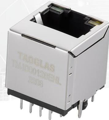
Featuring a popular footprint and compatible package to industry RJ45 Integrated Connectors standards, the Taoglas TMJD0012BENL is an RJ45 Integrated Connector 10/100Base-T Single Port and Vertical with shielded body and with a schematic that enables AutoMDIX feature.
