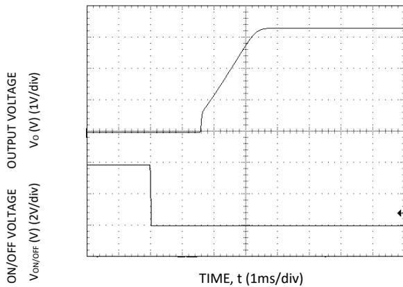
Figure 29. Typical Start-up Using On/Off Voltage (I<sub>o</sub> = I<sub>o,max</sub>).
