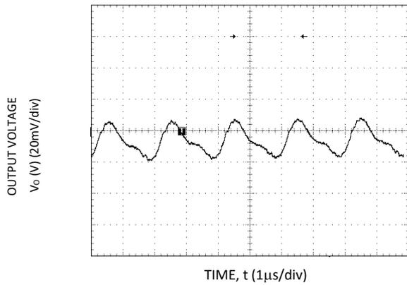
Figure 27. Typical output ripple and noise (V<sub>IN</sub> = 12V, I<sub>o</sub> = I<sub>o,max</sub>).
